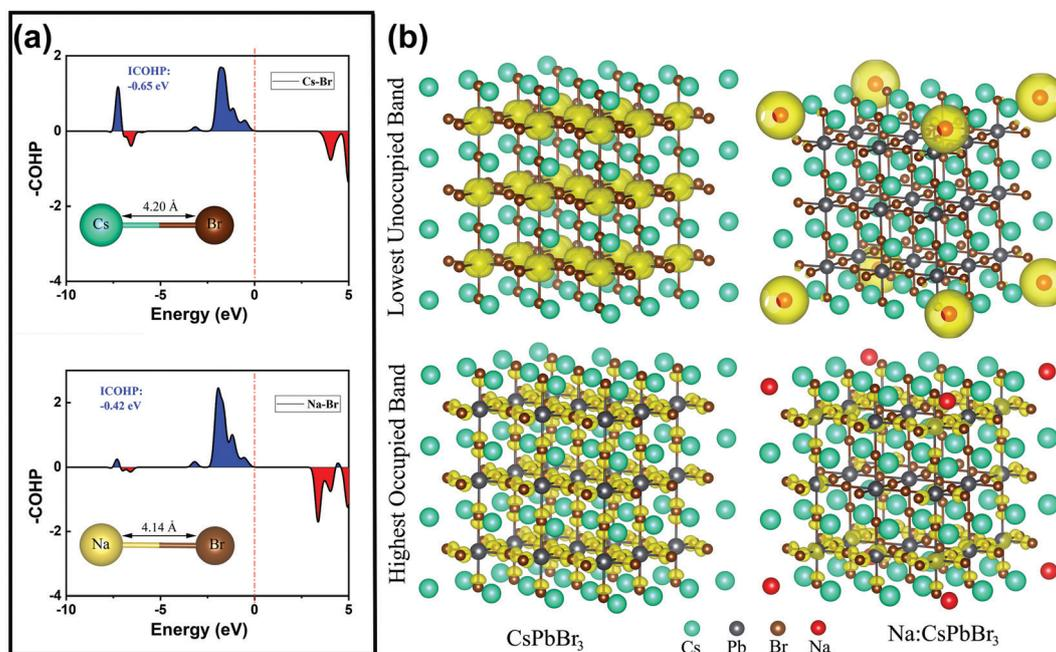
**Fig. 5** (a) COHP plots of Cs–Br and Na–Br interactions for CsPbBr<sub>3</sub> (top) and Na<sup>+</sup>-doped CsPbBr<sub>3</sub> (bottom). (b) The corresponding isosurfaces of the charge density of the highest occupied band (bottom) and lowest unoccupied band (top) in CsPbBr<sub>3</sub> and Na<sup>+</sup>-ion-doped CsPbBr<sub>3</sub>.
