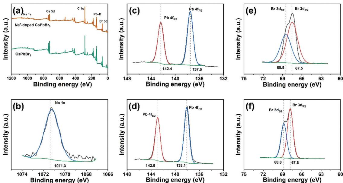
Fig. 3 (a) Survey XPS spectra of CsPbBr<sub>3</sub> and Na<sup>+</sup>-doped CsPbBr<sub>3</sub> QDs (Na/Cs = 1/3). (b) The high-resolution XPS spectrum of the Na 1s signal in the Na<sup>+</sup>-doped CsPbBr<sub>3</sub> QDs. (c–f) High-resolution XPS spectra corresponding to the Pb and Br elements in doped and undoped CsPbBr<sub>3</sub> QDs. The black curves represent the original data, the blue and red curves are the fitting peaks, and the green lines are the background.
