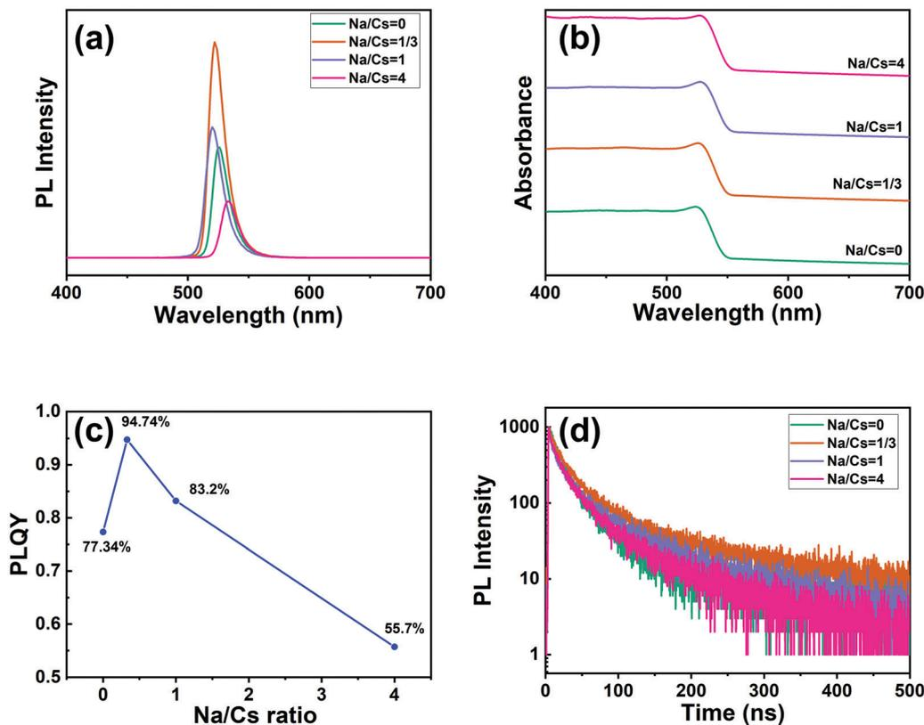
Fig. 4 (a) PL spectra (excited by 365 nm light), (b) absorption spectra, (c) PLQY data, and (d) time-resolved PL decay curves of CsPbBr<sub>3</sub> and Na<sup>+</sup>-doped CsPbBr<sub>3</sub> QDs.
