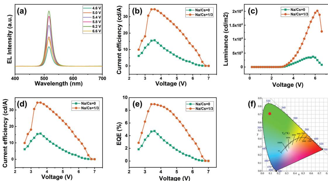
Fig. 7 (a) EL spectra of the Na<sup>+</sup>-doped CsPbBr<sub>3</sub> QD-based QLED device under different driving voltages. (b) Current density–voltage, (c) luminance–voltage, (d) current efficiency–voltage, and (e) EQE–voltage plots of the QLED device with undoped and Na<sup>+</sup>-doped CsPbBr<sub>3</sub> QDs as the emitting layer. (f) The chromaticity coordinates of the corresponding Na<sup>+</sup>-doped CsPbBr<sub>3</sub> QLED device.
