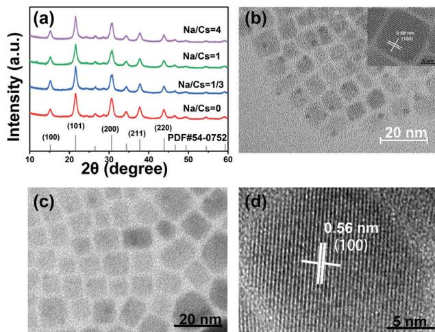
Fig. 2 (a) XRD patterns of the as-synthesized Na<sup>+</sup>-doped CsPbBr<sub>3</sub> QDs with different Na/Cs ratios. TEM images of (b) CsPbBr<sub>3</sub> and (c) representative Na<sup>+</sup>-doped CsPbBr<sub>3</sub> QDs (Na/Cs = 1/3). (d) A HRTEM image of a typical Na<sup>+</sup>-doped CsPbBr<sub>3</sub> QD. The inset of (b) shows a HRTEM image of one CsPbBr<sub>3</sub> QD.
