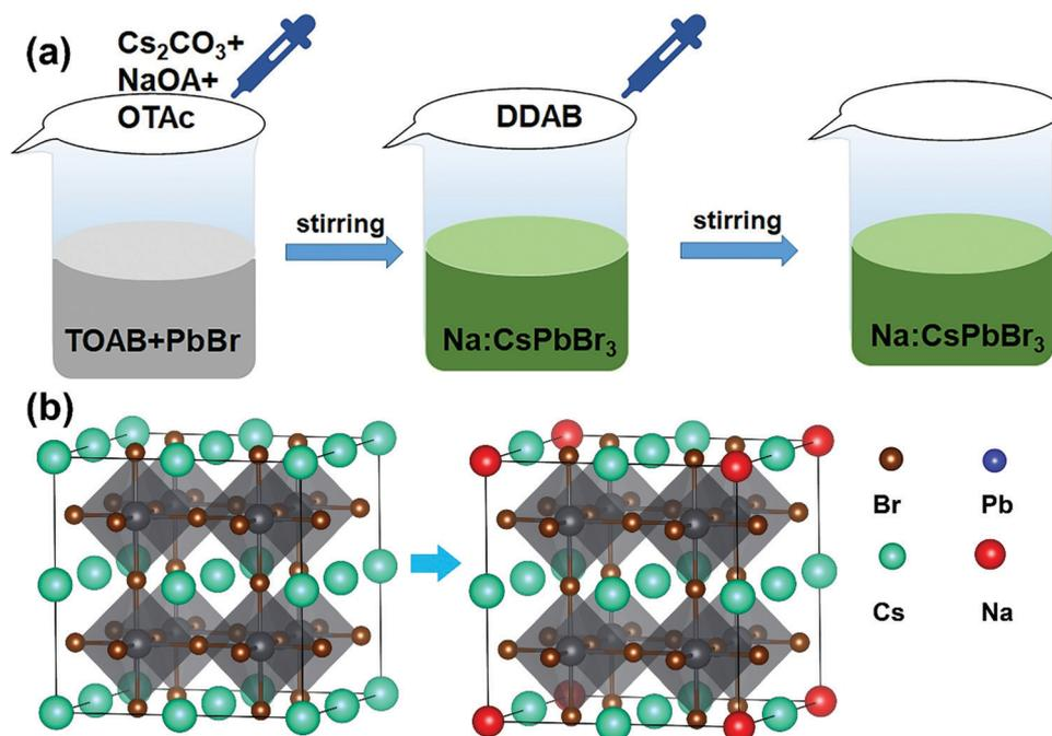
Fig. 1 (a) A schematic illustration of the synthesis procedure of  $\text{Na}^+$ -doped  $\text{CsPbBr}_3$  QDs. (b) A representative model of  $\text{Na}^+$ -doped  $\text{CsPbBr}_3$  QDs showing the replacement of some Cs positions with Na atoms.
