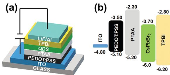
Fig. 6 (a) A schematic illustration and (b) flat-band energy level diagram of the CsPbBr<sub>3</sub> QLED device.
