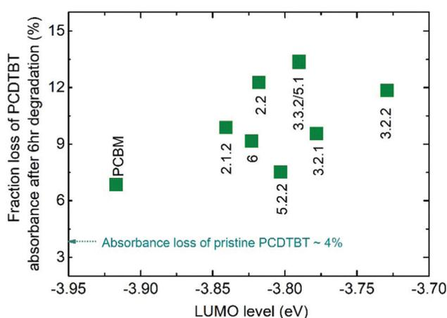
**Fig. 2** Fraction of initial polymer absorbance at 571 nm that is lost after 6 h exposure to AM 1.5G illumination in air for each PCDTBT:fullerene blend films as a function of the measured LUMO level of the acceptor. Also indicated is the absorbance loss of the pure polymer film. The absorbance measurements of neat fullerene films are not shown since there was no significant change after 6 h illumination, in agreement with results in the literature.<sup>30</sup>
