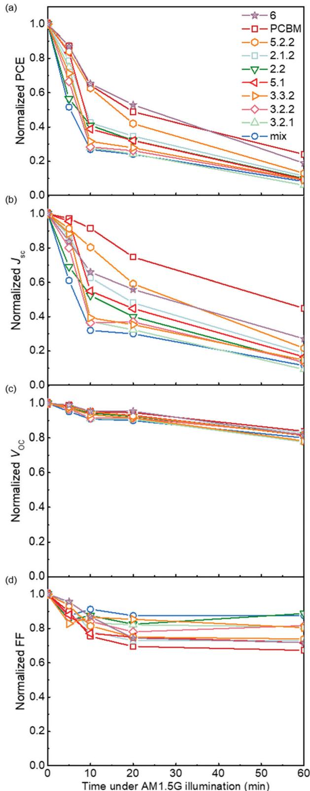
Fig. 3 Photovoltaic parameters (a) power conversion efficiency (PCE), (b) short circuit current density  $J_{sc}$ , (c) open circuit voltage  $V_{oc}$  and (d) fill factor FF of PCDTBT:fullerene devices as a function of the time for which the active layer had been exposed to simulated AM 1.5G illumination in air prior to electrode deposition. All performance parameters are normalised to the value measured for a device whose active layer was not exposed to air.
