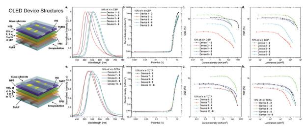
Fig. 5 The characteristics of the OLED devices. (a and e) Electroluminescence spectra. (b and f) Current density-bias characteristics. (c and g) EQE-current density characteristics. (d and h) EQE-luminance characteristics.
