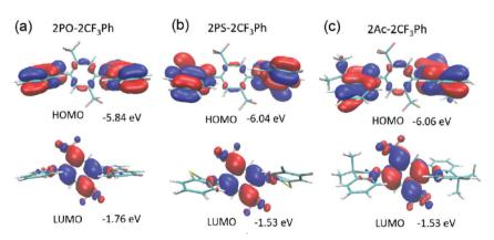
Fig. 2 HOMO and LUMO along with their energy levels for (a) 2PO-2CF<sub>3</sub>Ph, (b) 2PS-2CF<sub>3</sub>Ph and (c) 2Ac-2CF<sub>3</sub>Ph. Note there is no total separation of HOMO and LUMO electron clouds.
