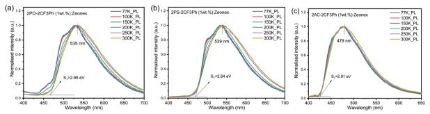
Fig. 5 The low-temperature and room-temperature PL of 2PO-2CF<sub>x</sub>Ph (a), 2PS-2CF<sub>x</sub>Ph (b) and 2AC-2CF<sub>x</sub>Ph (c) in Zeonex and the corresponding onsets of emission at 300 K.
