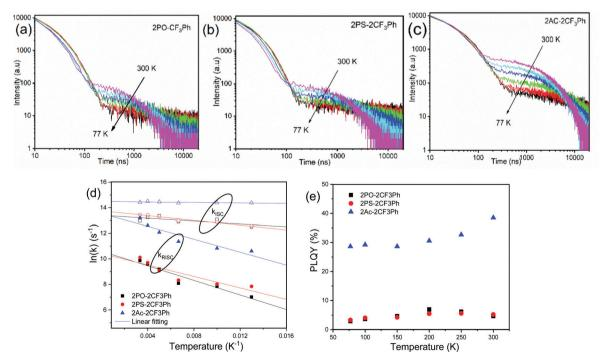
Fig. 6 Fluorescence decay of (a) 2PO-2CF<sub>3</sub>Ph (b) 2PS-2CF<sub>3</sub>Ph and (c) 2Ac-2CF<sub>3</sub>Ph doped 1 wt% in Zeonex as a function of temperature as well as their  $k_{\rm ISC}/k_{\rm RISC}$  (d) and PLQY (e) temperature dependences
