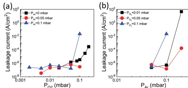
Fig. 4 (a) Leakage current at 1 V as a function of  $P_{\text{O}_2}$  for  $P_{\text{Ar}} = 0$  mbar (black squares, data reported in ref. 16),  $P_{\text{Ar}} = 0.05$  mbar (red circles) and  $P_{\text{Ar}} = 0.1$  mbar (blue triangles). (b) Leakage current at 1 V as a function of  $P_{\text{Ar}}$  for  $P_{\text{O}_2} = 0.01$  mbar (black squares), 0.05 mbar (red circles), and 0.1 mbar (blue up-pointing triangles).
