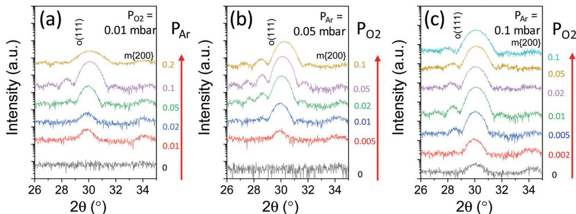
Fig. 1 XRD  $\theta$ - $2\theta$  scans of films deposited under a mixed Ar/O<sub>2</sub> atmosphere. (a) Fixed  $P_{O_2} = 0.01$  mbar and varying  $P_{Ar}$ . The scan corresponding to  $P_{Ar} = 0$  mbar and  $P_{O_2} = 0.01$  mbar has been reported in ref. 16. (b) Fixed  $P_{Ar} = 0.05$  mbar and varying  $P_{O_2}$ . (c) Fixed  $P_{Ar} = 0.1$  mbar and varying  $P_{O_2}$ .
