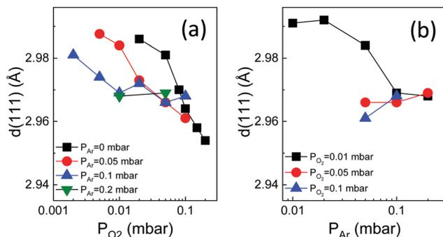
Fig. 3 Out-of-plane lattice parameter,  $d_{\text{HZO}(111)}$ , as a function of  $P_{\text{O}_2}$  (a) and  $P_{\text{Ar}}$  (b). In (a)  $P_{\text{Ar}}$  is 0 mbar (black squares, data reported in ref. 16), 0.05 mbar (red circles), 0.1 mbar (blue up-pointing triangles), and 0.2 mbar (green down-pointing triangles). In (b)  $P_{\text{O}_2}$  is 0.01 mbar (black squares), 0.05 mbar (red circles), and 0.1 mbar (blue up-pointing triangles).
