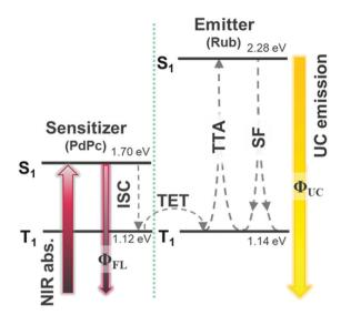
Fig. 1 TTA-UC energy scheme of Rub/PdPc with the corresponding energy transfer processes. ISC - intersystem crossing, TET - triplet energy transfer, TTA - triplet-triplet annihilation, SF - singlet fission, UC upconversion.
