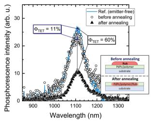
Fig. 4 PdPc phosphorescence spectra of the cold-deposited UC film before (circles) and after (triangles) annealing, and of the reference emitter-free film (solid line). TET{PdPc → Rub} efficiency of the untreated as well as annealed film is indicated. The inset schematically illustrates the UC film before and after annealing
