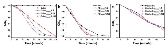
Fig. 4 Extents of methyl orange photodegradation with respect to the irradiation time for pristine and 2E-6MN-functionalized Cu<sub>2</sub>O (a) cubes, (b) rhombic dodecahedra, and (c) octahedra.
