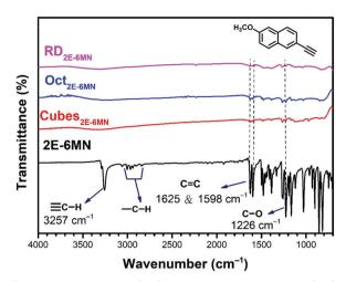
Fig. 3 FT-IR spectra of 2E-6MN molecules and the 2E-6MNfunctionalized Cu<sub>2</sub>O cubes, octahedra, and rhombic dodecahedra. The molecular structure is also shown
