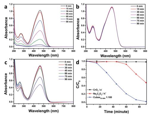
Fig. 5 UV-vis absorption spectra of methyl orange as a function of irradiation time using (a) 1:100 2E-6MN-modified Cu<sub>2</sub>O cubes as the photocatalyst and in the presence of (b) 3  $\mu$ mol of CrO<sub>3</sub> and (c) 3  $\mu$ mol of Na<sub>2</sub>C<sub>2</sub>O<sub>4</sub>. (d) Summary of the electron and hole scavenger tests.
