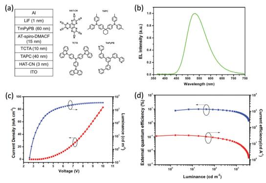
Fig. 5 Non-doped device performance for AT-spiro-DMACF: (a) device configuration and molecular structures of used materials; (b) EL spectrum at 5 V; (c) current density-voltage-luminance characteristics; and (d) EQE and current efficiency as a function of luminance.
