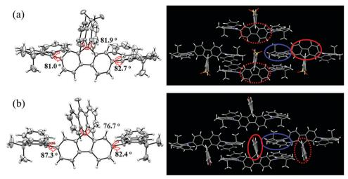
Fig. 2 Crystal structure and packing in TXADO-spiro-DMACF (a) and AT-spiro-DMACF (b). To indicate the possible CT route between the HOMO and the LUMO, the partial moieties are circled with blue and red solid lines (favorable) or dotted lines (unfavorable), respectively.
