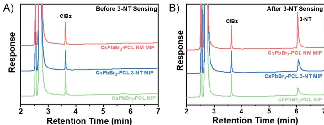
Fig. 6 Gas chromatograms of the CsPbBr<sub>3</sub>-PCL NIP and CsPbBr<sub>3</sub>-PCL 3-NT and NM MIP sensors (A) before and (B) after exposure to 3-NT vapours for 180 s.
