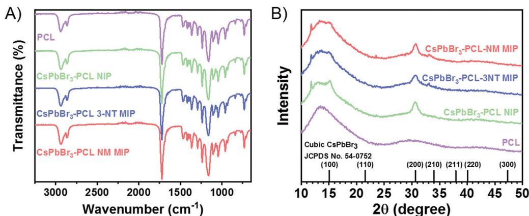
Fig. 2 (A) FTIR and (B) XRD spectra for PCL, CsPbBr<sub>3</sub>-PCL NIP, CsPbBr<sub>3</sub>-PCL 3-NT MIP, and CsPbBr<sub>3</sub>-PCL NM MIP.
