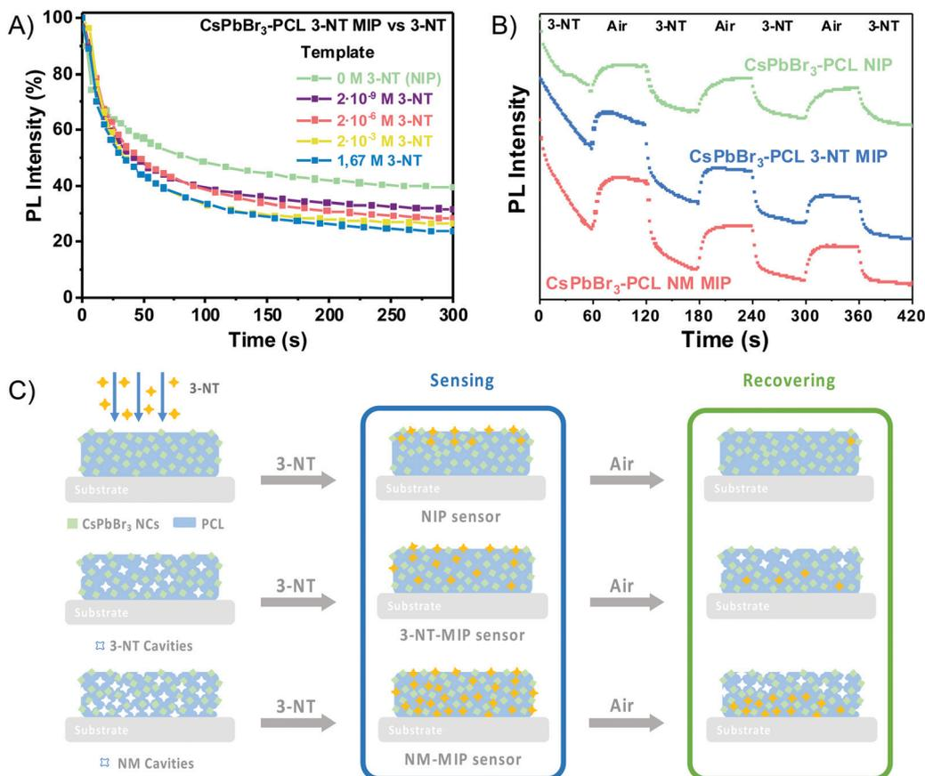
Fig. 5 (A) Real-time response of the CsPbBr<sub>3</sub>-PCL nanocomposite imprinted with different concentrations of 3-NT upon exposure to 3-NT vapours. (B) Real-time response of the CsPbBr<sub>3</sub>-PCL NIP and CsPbBr<sub>3</sub>-PCL 3-NT and NM MIP sensors under repeated exposure cycles to 3-NT vapours (grey areas) and air (white areas). (C) Schematic representation of the NIP/MIP sensing process.
