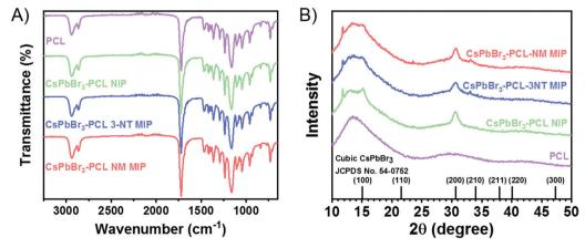
Fig. 2 (A) FTIR and (B) XRD spectra for PCL, CsPbBr<sub>3</sub>-PCL NIP, CsPbBr<sub>3</sub>-PCL 3-NT MIP, and CsPbBr<sub>3</sub>-PCL NM MIP.
