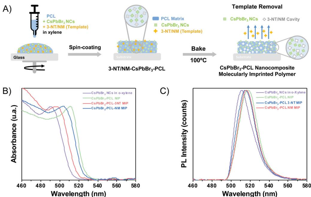
Fig. 1 (A) Schematic steps of the fabrication of the CsPbBr<sub>3</sub>-PCL 3-NT or NM MIP sensor. (B) UV-vis absorbance spectra and (C) emission spectra of CsPbBr<sub>3</sub> NCs in *o*-xylene (purple line) and embedded in the PCL polymer matrix without (green line), with 3-NT (blue line) and NM (red line) template.
