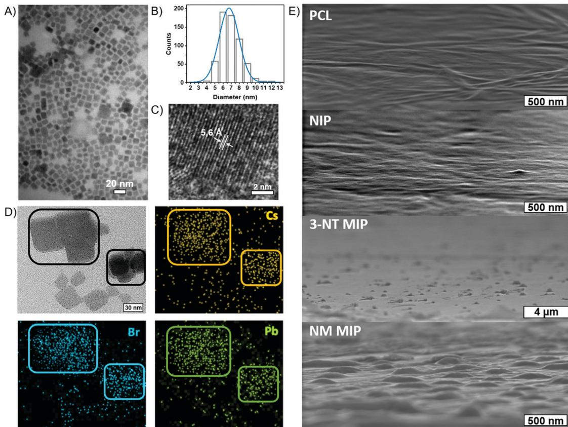
Fig. 3 (A) TEM image (B) size distribution of CsPbBr<sub>3</sub> NCs (C) HRTEM, and (D) HRTEM compositional mapping of CsPbBr<sub>3</sub>-PCL 3-NT MIP. (E) SEM images of the surface morphology of PCL, NIP, 3-NT MIP and NM MIP thin films.
