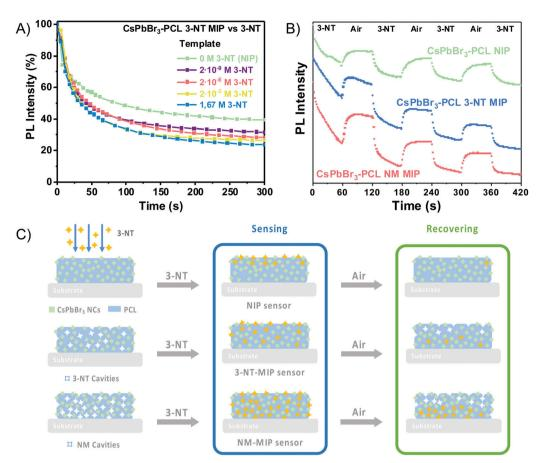
Fig. 5 (A) Real-time response of the CsPbBr<sub>3</sub>-PCL nanocomposite imprinted with different concentrations of 3-NT upon exposure to 3-NT vapours. (B) Real-time response of the CsPbBr<sub>3</sub>-PCL NIP and CsPbBr<sub>3</sub>-PCL 3-NT and NM MIP sensors under repeated exposure cycles to 3-NT vapours (grey areas) and air (white areas). (C) Schematic representation of the NIP/MIP sensing process.
