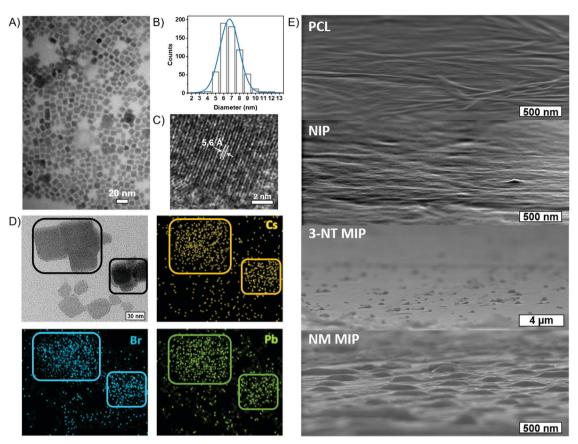
Fig. 3 (A) TEM image (B) size distribution of CsPbBr<sub>3</sub> NCs (C) HRTEM, and (D) HRTEM compositional mapping of CsPbBr<sub>3</sub>-PCL 3-NT MIP. (E) SEM images of the surface morphology of PCL, NIP, 3-NT MIP and NM MIP thin films.
