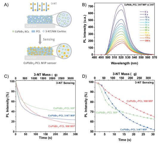
Fig. 4 (A) Schematic representation of the MIP sensing process. (B) Fluorescence response of the CsPbBr<sub>3</sub>-PCL 3-NT MIP sensor to 3-NT vapours. (C) Time- and 3-NT mass-dependent PL intensity of NIP, CsPbBr<sub>3</sub>-PCL 3-NT MIP and, CsPbBr<sub>3</sub>-PCL NM MIP nanocomposites sensing 3-NT and (D) PL intensity as a function of the amount of 3-NT and time exposure.
