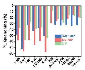
Fig. 7 Selectivity of the CsPbBr<sub>3</sub>-PCL sensor: 3-NT/NM MIP and NIP sensor response to different nitro-containing compounds and some common solvents after 180 s of exposure.
