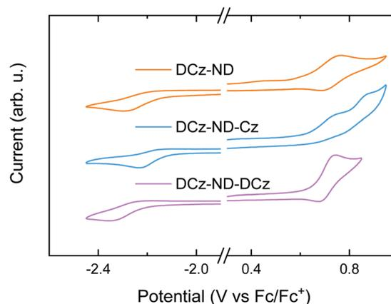
**Fig. 2** CV traces of the naphthyridine compounds in DMF under nitrogen with 0.1 M  $[n\text{-Bu}_4\text{N}]\text{BF}_4$  as the supporting electrolyte. Scan rate =  $50\text{ mV s}^{-1}$ ; compound concentration = 1 mM.
