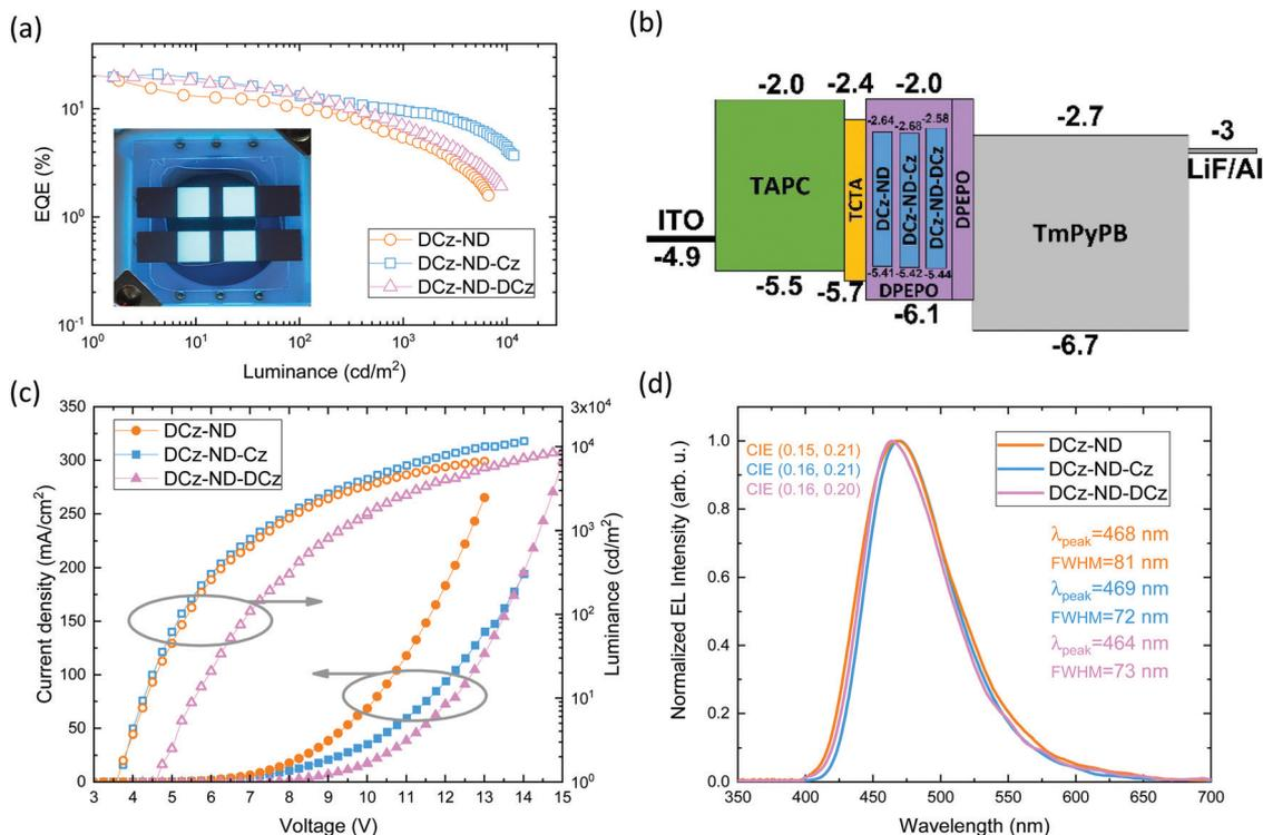
Fig. 5 Main characteristics of naphthridine-based TADF-OLEDs: (a) EQE vs. luminance with a picture of a working **DCz-ND-Cz** device in the inset; (b) energy level diagram; (c) current density and luminance vs. applied voltage; and (d) EL spectra at  $100 \text{ cd m}^{-2}$ .
