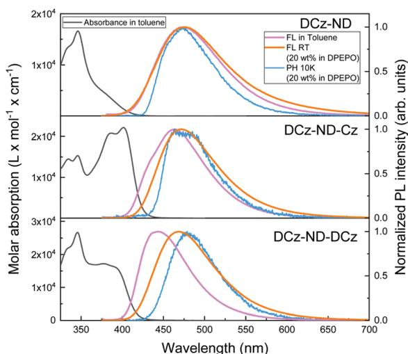
**Fig. 3** Absorption and fluorescence ( $1 \times 10^{-5}$  mol L<sup>-1</sup> in toluene), room-temperature fluorescence (20 wt% in DPEPO) and phosphorescence (20 wt% in DPEPO at 10 K, delay time 100  $\mu$ s) spectra of the carbazole–naphthyridine compounds **DCz-ND**, **DCz-ND-Cz** and **DCz-ND-DCz**.
