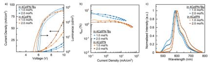
Fig. 4 (a) Comparison of current density-voltage-luminance (J-V-L) characteristics, (b) comparison of EQEs versus current densities, and (c) comparison of EL at EQE<sub>max</sub> for OLED with binary blend EML.
