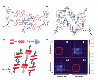
Fig. 2 (a and b) Crystal structures of DMAC-NZP and DMAC-NZC, respectively. (c) Schematic diagram of the discrete NZ dimer formation. (d) Transition density matrix color-filled map of the S<sub>1</sub> state of the DMAC-NZC dimer. The molecular conformation and crystal packing information are obtained by single-crystal X-ray diffraction (XRD)
