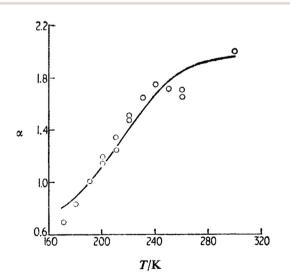
Fig. 5 Comparison of experiment and theory for the temperature dependence of  $\alpha$  (pyrene in ethanol): O, experiment, –, theory, =  $7 \times 10^{14}$  s<sup>-1</sup>, L = 0.17 nm, and B = 0.936. Reprinted (adapted) with permission.<sup>72</sup> Copyright 1989, Journal of Chemical Society.
