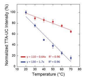
Fig. 9 Normalized TTA-UC emission intensity at 434 nm for the BSA/ SDS/1/DPA hydrogel and at 476 nm for the BSA/SDS/3/Pery hydrogel with respect to temperature. Reprinted (adapted) with permission. 88 Copyright 2020 American Chemical Society.
