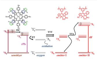
Fig. 3 Simplified energetic scheme of the triplet-triplet annihilation upconversion process in an oxygen rich environment. Inset: Chemical structures of the sensitizer - mixed palladium benzo- naphtho- porphyrins, n = 1, 0 (PdBNP); emitter – MPh-MB-BODI PY. Reprinted (adapted) with permission.<sup>68</sup> Copyright 2021 American Chemical Society.
