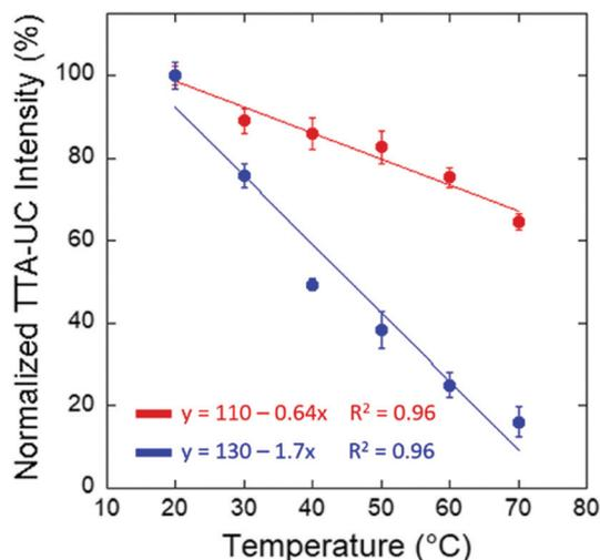
Fig. 9 Normalized TTA-UC emission intensity at 434 nm for the BSA/SDS/1/DPA hydrogel and at 476 nm for the BSA/SDS/3/Pery hydrogel with respect to temperature. Reprinted (adapted) with permission.<sup>88</sup> Copyright 2020 American Chemical Society.
