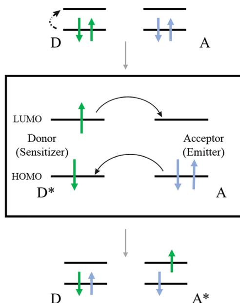
Fig. 4 Cartoon elucidating the Dexter energy transfer mechanism.
