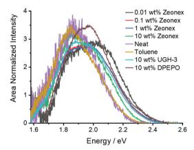
Fig. 4 Prompt fluorescence spectra (0.8 ns after excitation) extracted from the time-resolved emission decays of 4DTPIPN in the various solid films and in toluene solution at room temperature.
