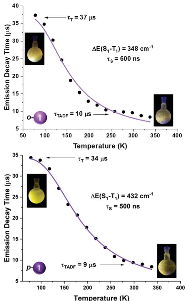
Fig. 8 Emission decay times of [Au(o-C<sub>6</sub>F<sub>4</sub>I)(dppBz)] (4) (top) and [Au(p-C<sub>6</sub>F<sub>4</sub>I)(dppBz)] (5) (bottom) versus temperature. The solid lines represent a fit of eqn (1) to the experimental data.
