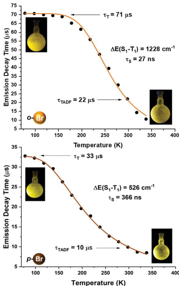
Fig. 7 Emission decay times of [Au(*o*-C<sub>6</sub>BrF<sub>4</sub>)(dppBz)] (2) (top) and [Au(*p*-C<sub>6</sub>BrF<sub>4</sub>)(dppBz)] (3) (bottom) versus temperature. The solid lines represent a fit of eqn (1) to the experimental data.
