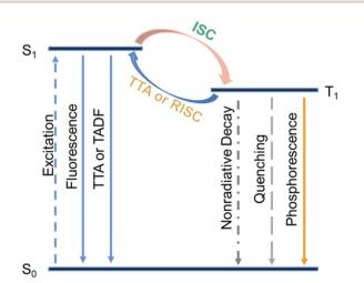
Scheme 1 Enhancing organic afterglow efficiency in dopant-matrix systems via TTA and TADF mechanisms.
