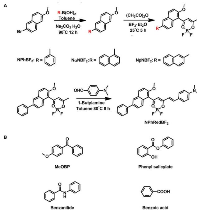
Scheme 2 Synthesis of naphthalene-containing BF<sub>2</sub>bdk luminescent compounds *via* a cascade reaction and further modification.
