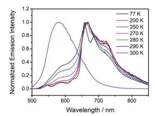
Fig. 5 Temperature-dependent delayed emission spectra NPhRedBF<sub>2</sub>-benzophenone samples.
