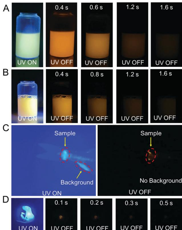
Fig. 7 (A) and (B) Photographs of (A)  $\text{N}\beta\text{NBF}_2\text{-MeOBP-0.5\%}$  and (B)  $\text{N}\beta\text{NBF}_2\text{-MeOBP-0.5\% + R6G}$  afterglow dispersion under 365 nm UV light and after removal of the UV light. (C) and (D) Preliminary bioimaging studies of the  $\text{N}\beta\text{NBF}_2\text{-MeOBP-0.5\%}$  afterglow dispersion in living (C) fish and (D) mice.
