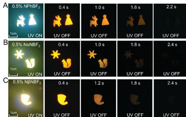
Fig. 2 Photographs of (A) NPhBF<sub>2</sub>–MeOBP-0.5%, (B) NαNBF<sub>2</sub>–MeOBP-0.5% and (C) NβNBF<sub>2</sub>–MeOBP-0.5% afterglow materials under 365 nm UV light and after removal of the UV light.
