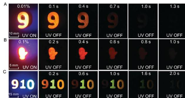
Fig. 6 Photographs of afterglow objects with desired shapes prepared by the melt casting technique of (A) NPhRedBF<sub>2</sub>-MeOBP-0.01%, (B) NPhRedBF<sub>2</sub>-MeOBP-0.1% and (C) (left–right) NPhRedBF<sub>2</sub>-MeOBP-0.01%, N $\alpha$ N-MeOBP-0.5% and N $\beta$ NBF<sub>2</sub>-MeOBP-0.5% under 365 nm UV light and after removal of the UV light.
