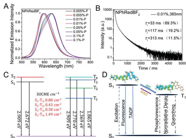
**Fig. 4** (A) Room-temperature steady-state emission and delayed emission spectra of NPhRedBF<sub>2</sub>-MeOBP afterglow materials at different doping concentrations. (B) Room-temperature emission decay of NPhRedBF<sub>2</sub>-MeOBP-0.01% afterglow materials excited at 365 nm and monitored at 599 nm. (C) and (D) Schematic representations of (C) energy levels and spin orbital coupling matrix elements and (D) the proposed mechanism of organic afterglow in the NPhRedBF<sub>2</sub>-MeOBP system.
