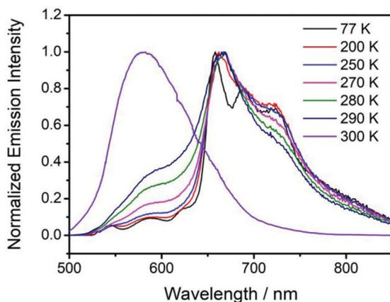
Fig. 5 Temperature-dependent delayed emission spectra of NPhRedBF<sub>2</sub>-benzophenone samples.
