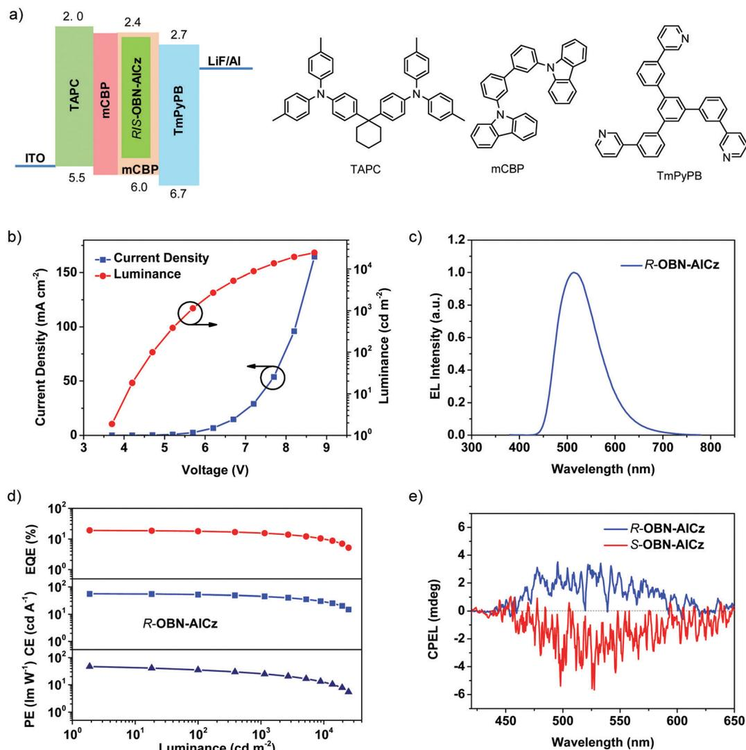
Fig. 5 (a) Device structure, energy level diagram and molecular structures of the materials employed in the optimized devices. (b) Current density–voltage–luminance ( $J$ – $V$ – $L$ ) characteristics, (c) EL spectra, and (d) efficiency–luminance characteristics of the optimized *R/S*-OBN-AICz-based OLEDs. (e) CPL spectra of the CP-OLEDs based on *R*-OBN-AICz and *S*-OBN-AICz.
