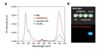
Fig. 2 (A) Emission spectra of each sample under 635 nm laser irradiation. A 632 nm notch filter was used to eliminate the scattered incident light. (B) Photographs of PCL, PdTPBP PCL, perylene PCL, and UC PCL under white light (top images) and 625 nm LED excitation (bottom images, 23.3 mW cm $^{-2}$ ), acquired through a 500 nm shortpass filter.
