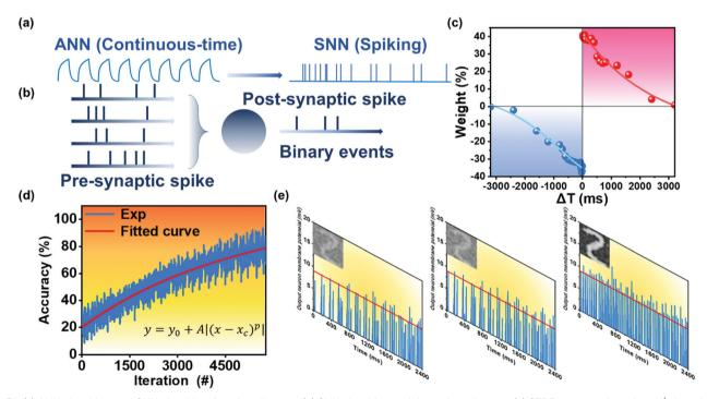
Fig. 5 (a) ANN algorithm and SNN algorithm function diagram. (b) SNN algorithm weight update diagram. (c) STDP response based on  $K^+$  doped  $AlO_x$ synaptic devices. (d) Image recognition rate of SNN algorithm. (e) Different stage results of training the SNN using the MNIST data set. Via the generation characteristics of the SNN, the image is reconstructed using the training weights connected to each output neuron to view the learning situation of the network
