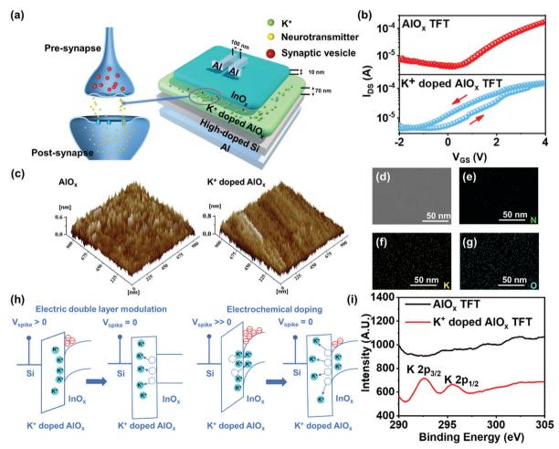
Fig. 1 (a) Schematic diagram of the  $K^+$  doped  $AlO_x$  synaptic TFT. (b) Transmission characteristics of  $AlO_x$  with and without  $K^+$  doped. (c) AFM images of  $AlO_x$  with and without  $K^+$  doped. (d) SEM image of surface topography in  $AlO_x$  surface view. The EDS mapping of (e) N, (f) K, (g) O elements in  $AlO_x$  coating on Si substrate. (h)  $K^+$  ions migration in the  $K^+$  doped  $AlO_x$  solid-state electron by bias spikes. (i) XPS image of the surface  $InO_x$  film.
