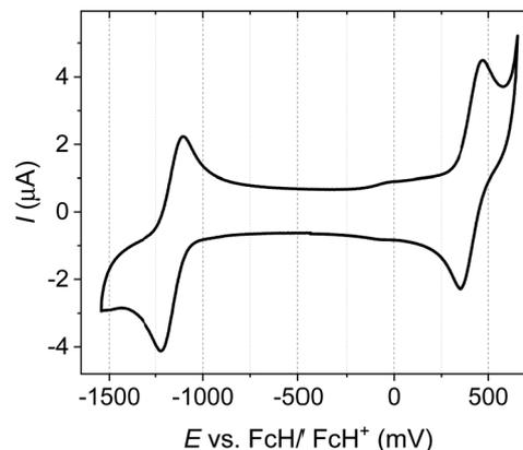
Fig. 3 Cyclic voltammogram recorded for **CAT-TPE** with 0.1 M *n*-Bu<sub>4</sub>NPF<sub>6</sub> in THF as the supporting electrolyte (scan rate = 100 mV s<sup>-1</sup>).
