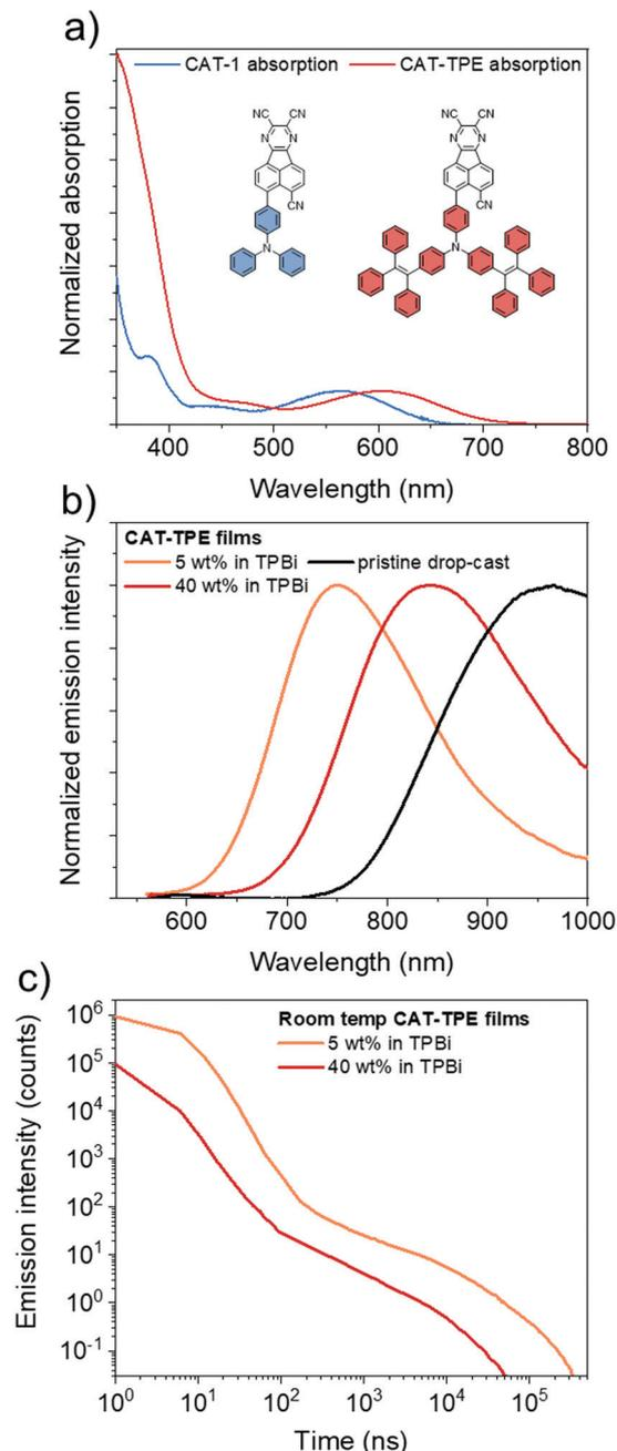
Fig. 2 (a) Absorption spectra of **CAT-1** and **CAT-TPE** in toluene solution; (b) photoluminescence spectra of **CAT-TPE** films ( $\lambda_{\text{exc}} = 405$  nm); (c) integrated photoluminescence kinetics of **CAT-TPE** films under vacuum ( $\lambda_{\text{exc}} = 400$  nm,  $10^{-5}$  mbar).
