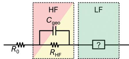
Fig. 8 General structure of the proposed ECM.  $R_0$  accounts for the Ohmic resistance of the contacts and current collectors,  $C_{\text{geo}}$  is the geometrical capacity,  $R_{\text{HF}}$  is the sum of all HF features in the spectrum and the LF-ECM will be detailed below.
