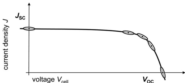
Fig. 5 Schematic of a  $JV$  curve with possible operating points for IS measurements,  $V_{OC}$ ,  $J_{SC}$  and MPP plus around the MPP. The points within the ellipses signify the essential steady-state operating point and the ellipses themselves indicate the range of voltage and current density that the devices undergo during the IS measurement, respectively.
