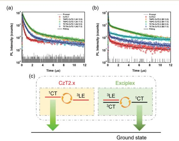
Fig. 4 Time-resolved photoluminescence (TRPL) decay curves of (a) CzT2.1 neat film and A1, A2 blend films and (b) CzT2.2 neat film and B1, B2 blend films, and (c) schematic representation of the emission mechanisms of the D:A blends.
