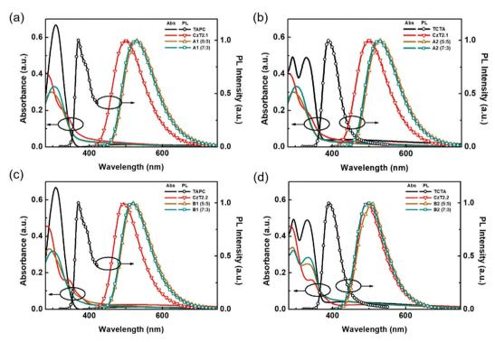
Fig. 3 UV-Vis absorption and PL spectra of the respective donors, acceptors, and D:A blend films (a) A1, (b) A2, (c) B1, and (d) B2.
