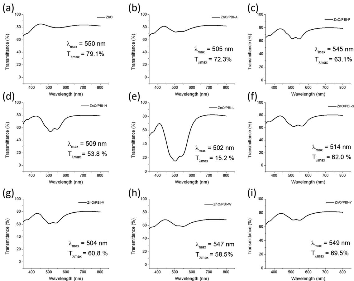
Fig. 2 Transmittance spectra of (a) ITO/ZnO and ITO/ZnO/PBI films where the PBI material used is (b) **PBI-A** (38 nm), (c) **PBI-F** (26 nm), (d) **PBI-H** (71 nm), (e) **PBI-L** (264 nm), (f) **PBI-S** (38 nm), (g) **PBI-V** (37 nm), (h) **PBI-W** (66 nm), (i) **PBI-Y** (39 nm). Transmittance at  $\lambda_{\max}$  is reported for the visible region. The average thickness measured for the ZnO/PBI double layers are stated in parentheses.
