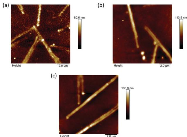
Fig. 4 AFM topography images of P3HT/PC<sub>61</sub>BM deposited on (a) ITO/ZnO/**PBI-A**, (b) ITO/ZnO/**PBI-F** and (c) ITO/ZnO.
