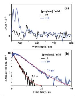
Fig. 3 (a) Transient absorption (TA) spectra at the time delay of 20  $\mu$ s and (b) decay time profiles of the TA signal at 490 nm, measured for Au<sub>2</sub>Cu<sub>6</sub> (270  $\mu$ M) with 0 and 10 mM perylene in deaerated THF at 298 K (excitation wavelength,  $\lambda_{ex} = 532$  nm).
