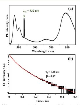
Fig. 4 (a) PL spectrum obtained for the deaerated THF solution of Au<sub>2</sub>Cu<sub>6</sub> (11  $\mu$ M) and perylene (5 mM), and (b) decay curve of the upconverted emission of perylene obtained by monitoring only the  $\lambda \leq$  492 nm region using short-pass filters. The fitting of the decay curve was performed using egn (1). The 532 nm-CW laser was used in these measurements. Note that the upconverted emission of perylene was also observed when using a 640 nm-CW laser.
