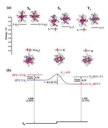
Fig. 7 (a) Computed energy-level diagram for the optimized structures of  $S_0, S_1$ , and  $T_1$  (lower panel). The electronic configuration of each electronic state is shown with upward (α-spin) and downward (β-spin) arrows in the notations HOMO (H), LUMO (L), and LUMO+1 (L+1). (b) Schematic representation of the ISC mechanism of the Au $_2$ Cu $_6$  cluster. All values are in eV. Numbers in italics are the calculated values, while other numbers are estimated from the experiments.
