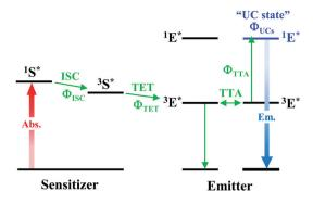
$\Phi_{\text{UCs}} = \Phi_{\text{ISC}} \cdot \Phi_{\text{TET}} \cdot \Phi_{\text{TTA}}$ Fig. 5 Schematic diagram of TF-UC occurring in the system of a sensi-
