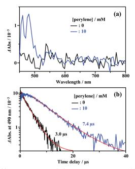
Fig. 3 (a) Transient absorption (TA) spectra at the time delay of 20  $\mu$ s and (b) decay time profiles of the TA signal at 490 nm, measured for Au<sub>2</sub>Cu<sub>6</sub> (270  $\mu$ M) with 0 and 10 mM perylene in deaerated THF at 298 K (excitation wavelength,  $\lambda_{ex} = 532$  nm).
