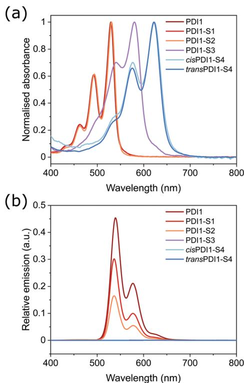
Fig. 1 UV/Vis absorbance spectra (a), and fluorescence spectra (b), of **PDI1**, **PDI1-S1**, **PDI1-S2**, **PDI1-S3**, **cisPDI1-S4**, **transPDI1-S4**, and **PDI1-S5**. All spectra recorded at a concentration of  $10^{-5}$  M in chloroform. Excitation wavelengths were chosen based on the maxima of the corresponding absorbance; 530 nm for **PDI1**, **PDI1-S1**, and **PDI1-S2**, 580 nm for **PDI1-S3**, 622 nm for **cisPDI1-S4** and **transPDI1-S4**, and 670 nm for **PDI1-S5**.
