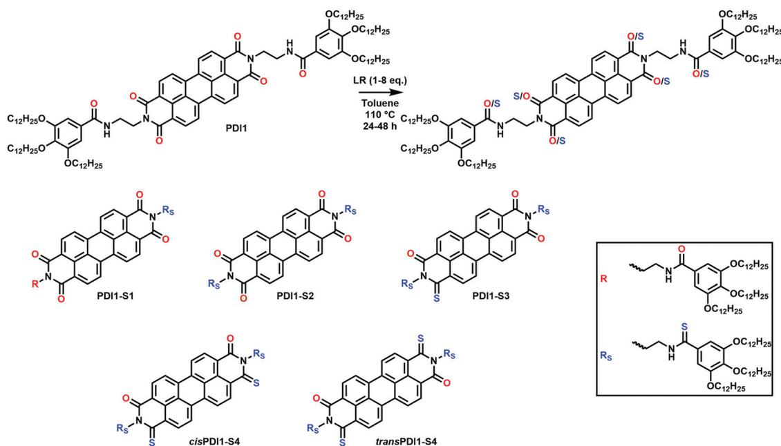
**Scheme 1** General conditions used for the thionation of **PDI-1** with Lawesson's reagent (LR). Chemical structures of products isolated from thionation with between one and four oxygen-to-sulphur substitutions.
