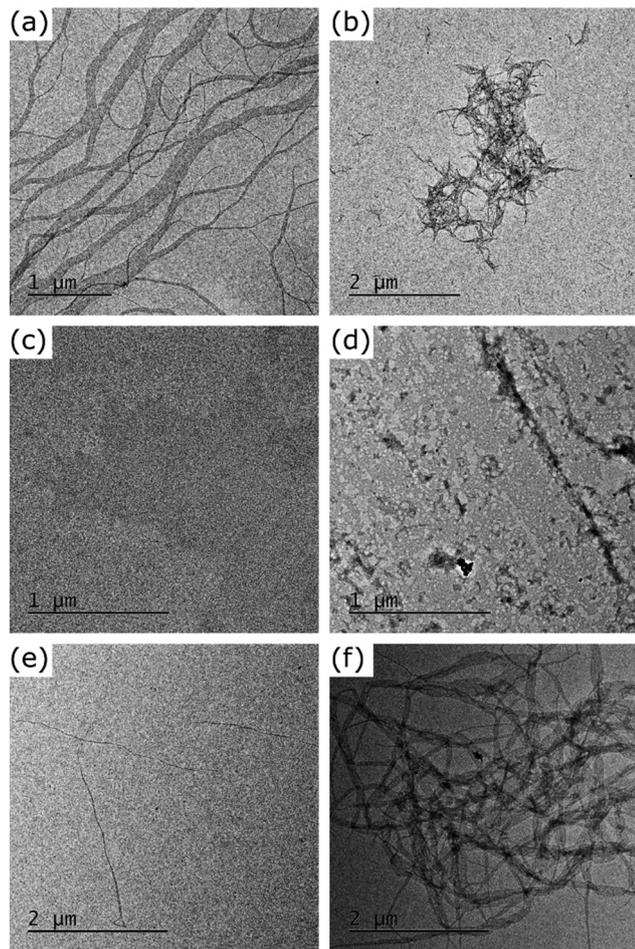
Fig. 2 TEM images of the morphologies formed by the self-assembly of **PDI1** (a), **PDI1-S1** (b), **PDI1-S2** (c), **PDI1-S3** (d), **cisPDI1-S4** (e), and **transPDI1-S4** (f), in MCH at a concentration of  $5 \times 10^{-5}$  M.
