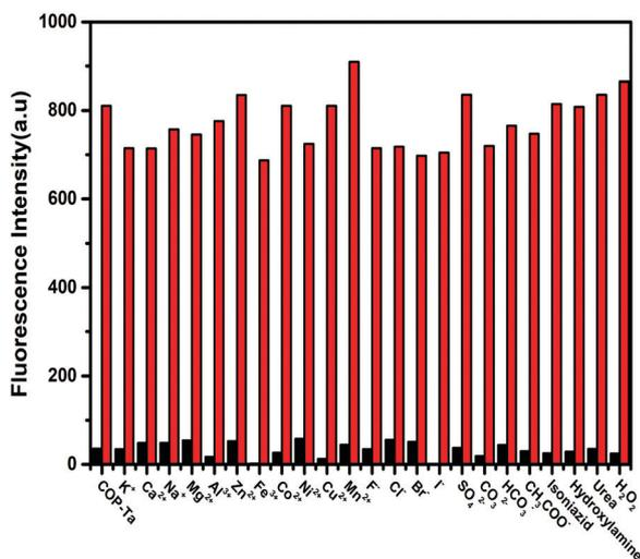
Fig. 5 Comparison of the fluorescence intensity of COP-Ta in the presence of various interfering components ( $100 \mu\text{M}$ ) in water before (black bar) and after (red bar) the addition of hydrazine ( $200 \text{ mM}$ ).
