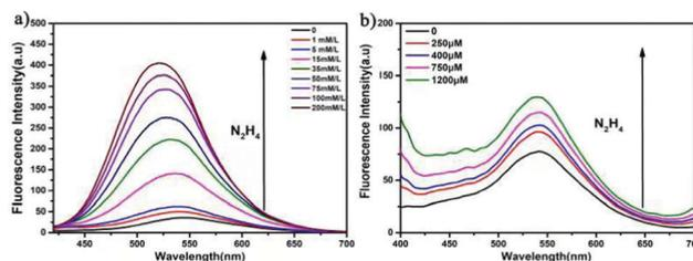
Fig. 6 Fluorescence response changes of COP-Ta in ethanol ( $0.6 \text{ mg mL}^{-1}$ ) toward hydrazine with various concentrations at room temperature in real water ( $\lambda_{\text{ex}} = 365$  nm) (a) and human blood serum. Experimental conditions:  $0.2 \text{ M}$  PBS buffer solution ( $\lambda_{\text{ex}} = 365$  nm) (b).
