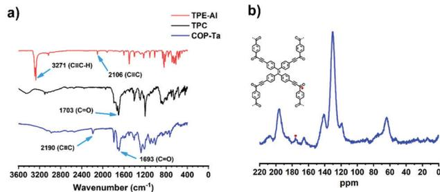
Fig. 1 (a) FT-IR spectra of TPE-Al, TPC and COP-Ta. (b) Solid-state <sup>13</sup>C CP-MAS NMR of COP-Ta.
