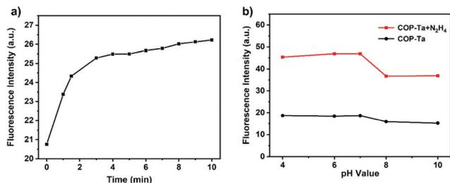
Fig. 4 (a) Time-dependent fluorescence changes of COP-Ta upon the addition of hydrazine ( $\lambda_{\text{ex}} = 365$  nm). (b) The effect of pH on the fluorescence intensity of COP-Ta with (red) and without (black) the addition of  $100 \mu\text{M}$  of hydrazine ( $\lambda_{\text{ex}} = 365$  nm).
