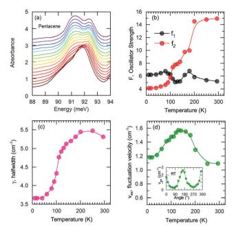
Fig. 5 (a) Temperature-dependent absorption spectra in the range of 90 meV, estimated energy range of the vibronic feature from the independent boson analysis for B and D. (b-d) Symbols represent the fit parameters of the Kubo formula, whereas the solid lines are guides to the eye. Inset in (d) is the angle dependence of the fluctuation velocity, which disappears when  $E \perp$  dimers.
