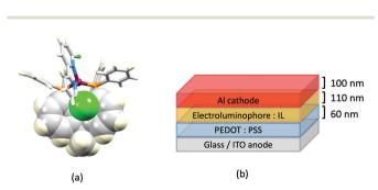
Fig. 10 (a) Structure of the cation in [Cu(xantphos)(6,6'-Cl<sub>2</sub>bpy)][PF<sub>6</sub>] (CSD refcode MEWXUK). (b) Architecture of LECs containing the Cu-iTMCs with halogen-substituted bpy ligands. IL = [EMIM][PF<sub>6</sub>] and Cu-iTMC: IL molar ratio = 4:1. LECs were driven using a pulsed current.
