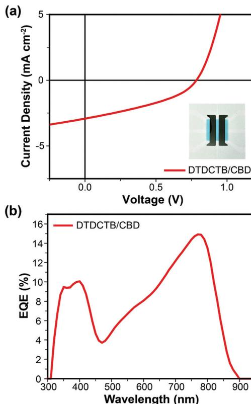
Fig. 2 (a)  $J$ – $V$  characteristics and (b) EQE curve for the optimal VD-SMSC based on DTDCTB and **CBD** under AM 1.5G ( $100 \text{ mW cm}^{-2}$ ) illumination. The inset graph in (a) is a photograph of the optimal device and the effective area is  $0.09 \text{ cm}^2$ .
