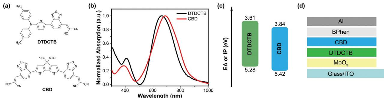
Fig. 1 (a) Molecular structures of the donor DTDCTB and the acceptor **CBD**. (b) UV-vis-NIR absorption spectra. (c) EA and IP of the DTDCTB and **CBD** films and (d) device structure of the VD-SMSCs based on DTDCTB and **CBD**.
