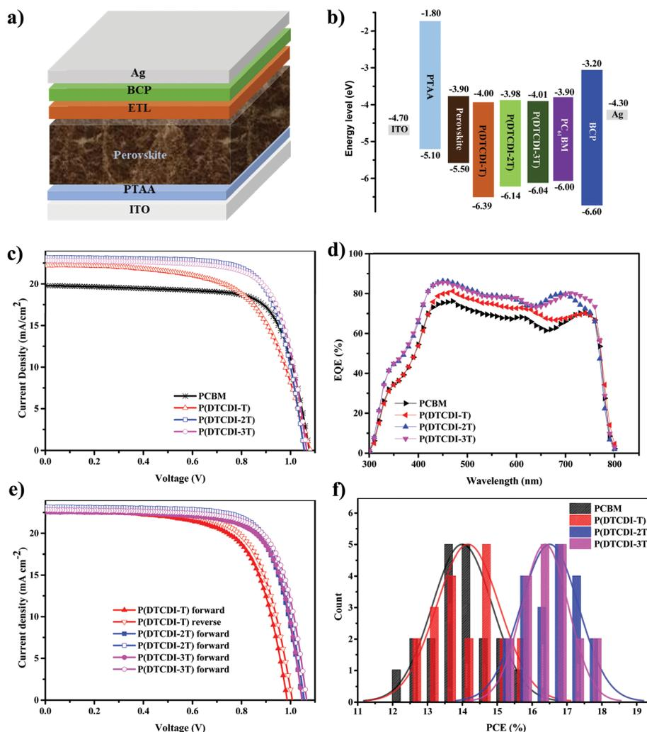
Fig. 2 (a) Schematic illustration of the device configuration. (b) Band alignment of PSCs with different ETLs. (c)  $J-V$  curves of PSCs with different ETLs and (d) EQE spectrum. (e)  $J-V$  hysteresis of optimal PSCs with P(DTCDI-T), P(DTCDI-2T) and P(DTCDI-3T) ETLs under forward and reverse scan. (f) Device efficiency distribution with different ETLs.
