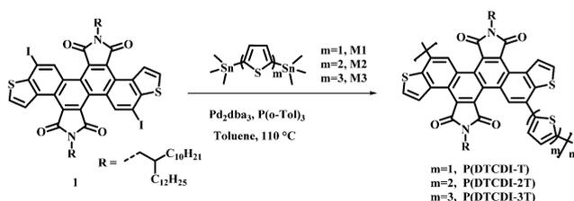
Scheme 2 Synthesis of P(DTCDI-T), P(DTCDI-2T) and P(DTCDI-3T).
