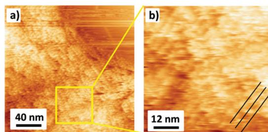
**Fig. 2** Ambient STM images show that the stacking phase of the DBV<sup>0</sup> film remains permanently intact after being disconnected from the electrochemical cell; tunneling parameters:  $V_b = -0.55$  V,  $I_t = 150$  pA.
