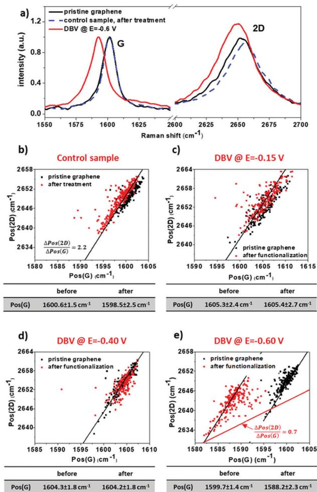
Fig. 4 (a) Raman spectra and (b–e) plots of Pos(2D) versus Pos(G) of G-SiO<sub>2</sub> samples before and after electrodeposition of DBV. The electrochemical potential at which G-SiO<sub>2</sub> is functionalized by DBV is indicated on top of the panels. The black lines in (b–e) have a slope of 2.2 and highlight the variation in strain and the red guideline in (e) indicates the direction in shift of the data points upon doping.
