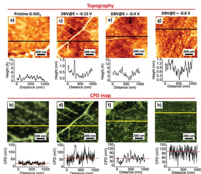
Fig. 3 AFM topographies (a, c, e and g) and corresponding CPD mappings (b, d, f and h) of DBV functionalized G-SiO<sub>2</sub>. The electrochemical potential at which G-SiO<sub>2</sub> is functionalized by DBV is indicated on top of the panels.
