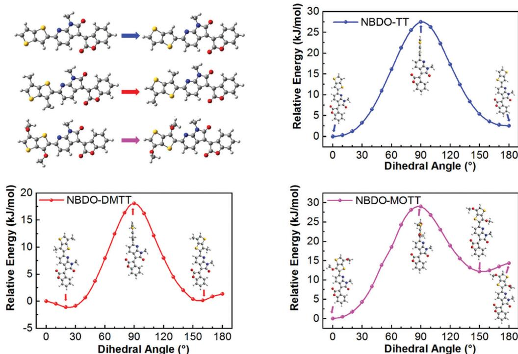
Fig. 3 Potential energy distribution of single-bond rotation in substructures of NBDO-based polymers with different substituents. Insets are corresponding conformers at local energy minima or maxima.
