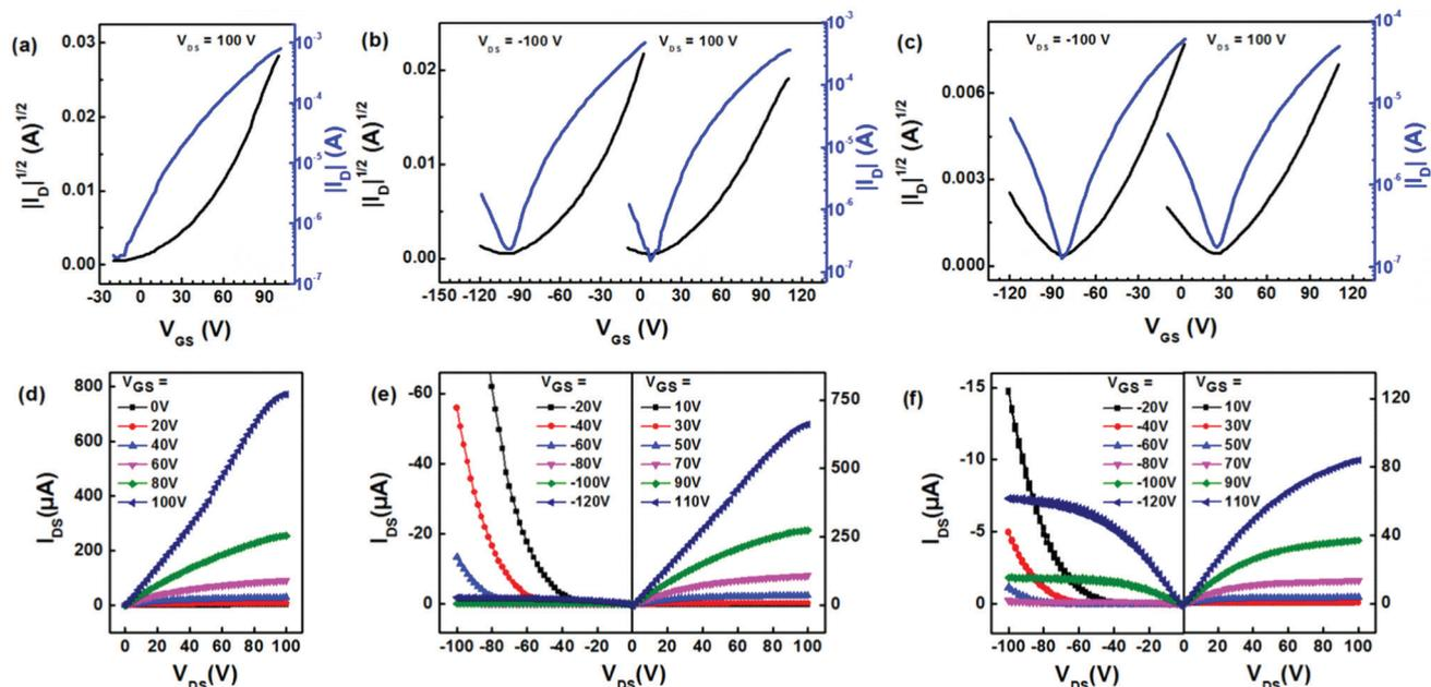
Fig. 4 The transfer (a–c) and output (d and f) characteristics of the field-effect transistors based on three polymers measured under optimized conditions. (a and d) **PNBDO-TT**. (b and e) **PNBDO-DMTT**. (c and f) **PNBDO-MOTT**.
