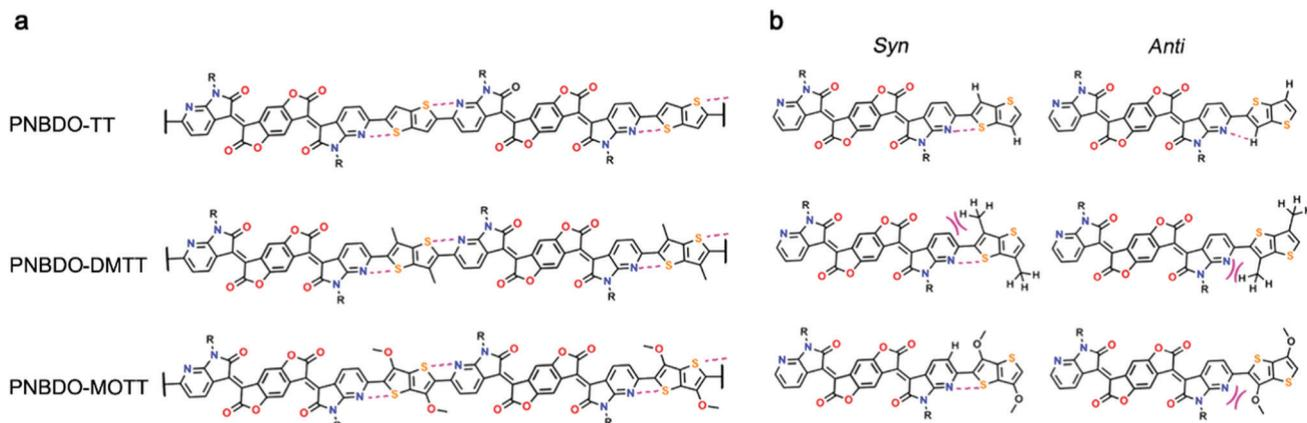
Fig. 2 Schematic illustration of noncovalent interactions and steric repulsions in the polymer system. (a) Dimeric co-repeating unit with  $S \cdots N$  interactions. (b) Different conformations of a co-repeating unit with noncovalent attractions or repulsions or both.
