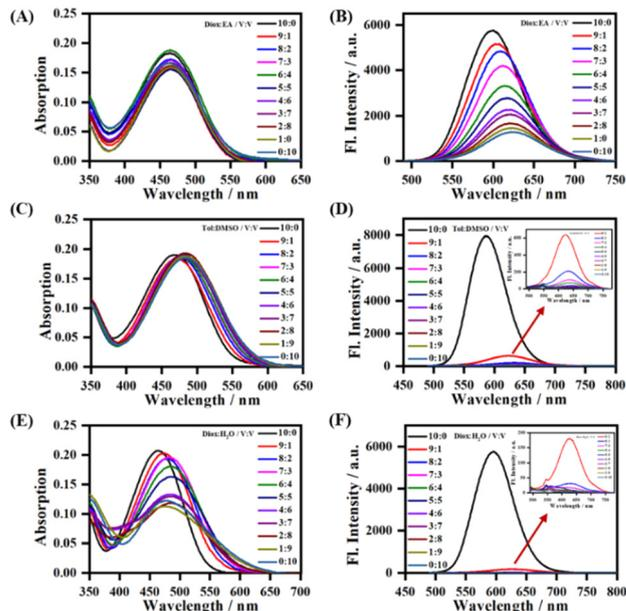
Fig. 2 The absorption (A, C and E) and fluorescence (B, D and F) spectra of **LDER** in 1,4-dioxane-EA, toluene-DMSO and 1,4-dioxane- $\text{H}_2\text{O}$  mixtures with different volume ratios; inset: the enlarged part indicated by the red arrow. Concentration = 10  $\mu$ M.
