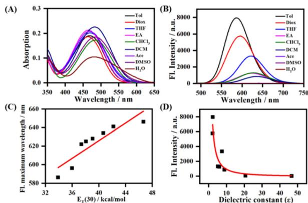
Fig. 1 The absorption (A) and fluorescence (B) spectra of **LDER** in different polarity solvents; (C) plot of the maximum wavelength of **LDER** with  $E_T(30)$ ; (D) fluorescence intensity change of **LDER** versus dielectric constant ( $\epsilon$ ). Concentration = 10  $\mu$ M. Solvents: Tol: toluene; Diox: 1,4-dioxane; THF: tetrahydrofuran; EA: ethyl acetate;  $\text{CHCl}_3$ : trichloromethane; DCM: dichloromethane; Ace: acetone; DMSO: dimethyl sulfoxide;  $\text{H}_2\text{O}$ : water.
