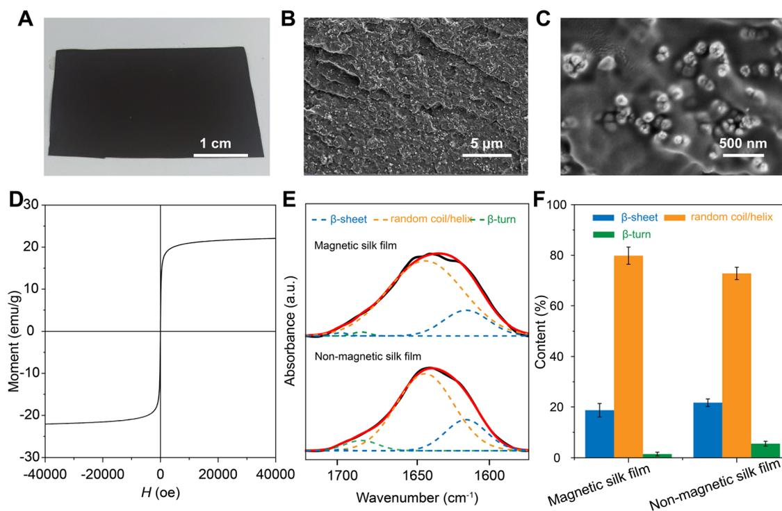
Fig. 3 (A) Photograph of the magnetic silk film. (B and C) SEM images of the magnetic silk film. (D) The magnetization curves of the Fe<sub>3</sub>O<sub>4</sub> particles at 37 °C. Inset: Close-up of the hysteresis at  $H = 0$ . (E) FTIR spectra of the magnetic and non-magnetic silk films. (F) Secondary structures of the silk proteins in the films from the deconvolution of the amide I region.
