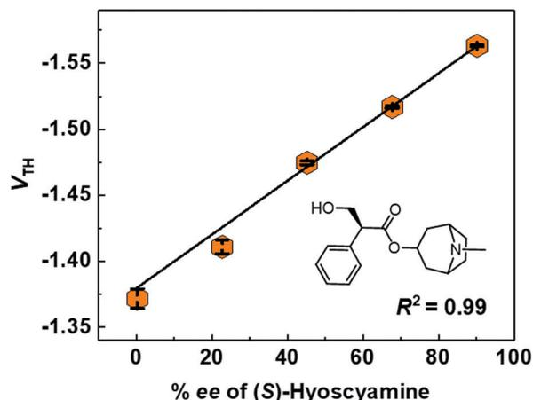
Fig. 7 Threshold voltage ( $V_{TH}$ ) corresponding to the % ee value of (*S*)-hyoscyamine in a phosphate buffer (100 mM, pH 7.0) containing KCl (100 mM) at 25 °C. The overall hyoscyamine concentration was set to 5.0  $\mu$ M.
