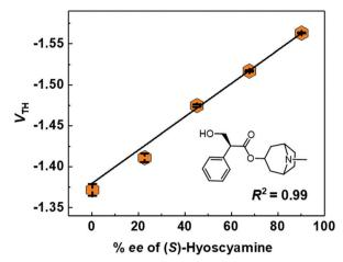
Fig. 7 Threshold voltage  $(V_{TH})$  corresponding to the % ee value of (S)hyoscyamine in a phosphate buffer (100 mM, pH 7.0) containing KCl (100 mM) at 25 °C. The overall hyoscyamine concentration was set to 5.0 µM.
