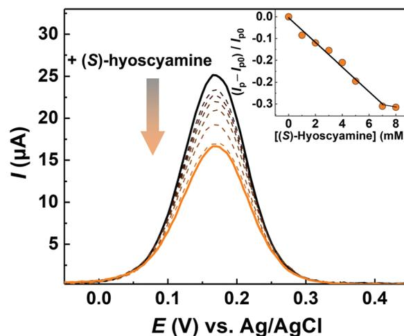
Fig. 4 DPV results of the MIP-AuNS electrode by adding (S)-hyoscyamine in a phosphate buffer (100 mM, pH 7.0) containing  $\text{K}_3\text{Fe}(\text{CN})_6$  (5 mM) and KCl (100 mM) at  $25\text{ }^\circ\text{C}$ . Inset represents the ratio of the peak current ( $I_p$ ) changes of the MIP-AuNS electrode upon adding (S)-hyoscyamine. The terms  $I_{p0}$  and  $I_p$  indicate the peak currents before and after adding (S)-hyoscyamine, respectively. [(S)-hyoscyamine] = 0.0–8.0 mM.
