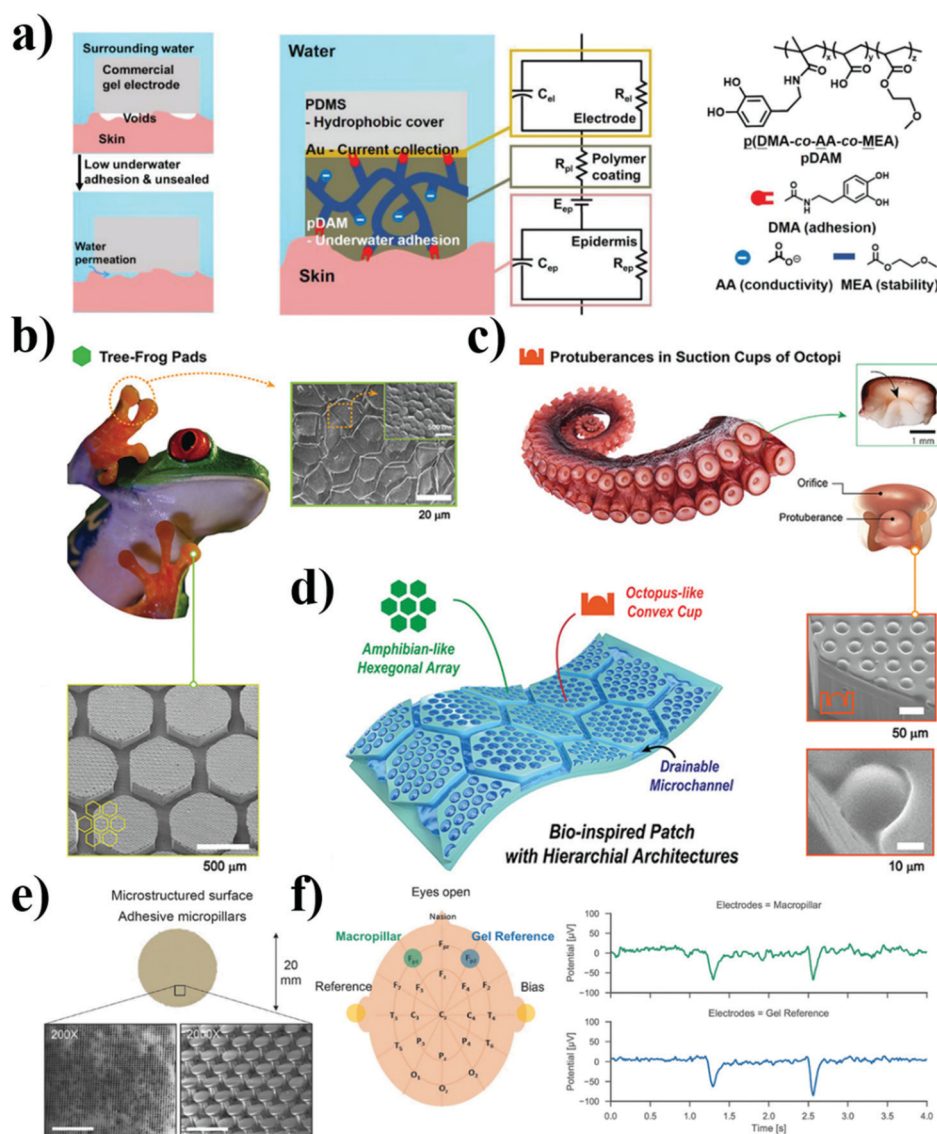
Fig. 6 Possible methods to improve the adhesion of EEG electrodes. (a) Voids exist at the commercial gel electrode–skin interface due to skin surface structure, which allows water in and cause decreased EEG adhesion. Schematic showing the water-resistant pDAM polymer coating bridging the Au/ Polydimethylsiloxane (PDMS) electrode and skin, and the corresponding circuit. Chemical structures of the dopamine-containing ionic-conductive random copolymer pDAM. 139 (b) Photograph of pads of a tree frog and scanning electron microscopy (SEM) images of hexagonal structures on its pads and the hierarchical structures (400 \mu m thickness, PDMS) of frog-inspired hexagonal microchannels (200 \mu m in width, 300 \mu m in height, and 600 \mu m spacing). (c) Photographic images of Octopus vulgaris tentacle and suction cup with protuberance and SEM images of the hierarchical structures with octopus-like convex structures (15 \mu m in radius and 18 \mu m in height) on hexagonal microchannels. (d) Schematic illustration of the amphibian and octopus-like hierarchical architectures. 142 (e) Soft electrode with grasshopper inspired microstructured surface for improved dry adhesion to the skin (thickness = 100 \mu m). The scale bars are 200 \mu m (200 \times ) and 20 \mu m (2000 \times ). (f) The alpha waves disappear when the eyes are kept open. The peaks in the time signal correspond to typical eye blink effects. 149
