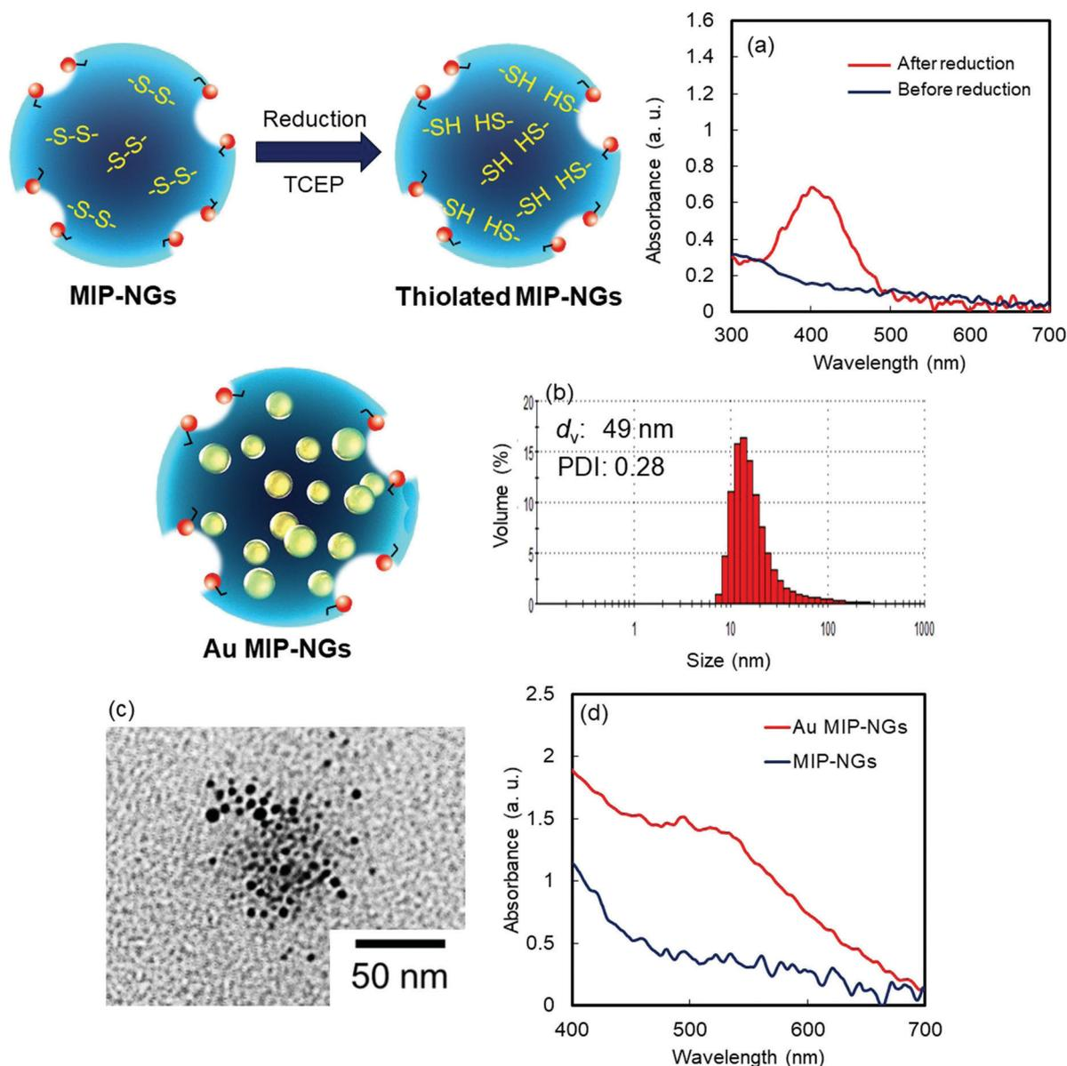
**Fig. 1** (a) DTNB assay for MIP-NGs before (blue) and after (red) the reduction of MIP-NGs using TCEP. (b) Particle size distribution measured using DLS and (c) TEM image of Au MIP-NGs. (d) UV-Vis spectra of the MIP-NGs before (blue) and after (red) the generation of Au NPs. TCEP: tris(2-carboxyethyl) phosphine; DLS: dynamic light scattering; TEM: transmittance electron microscopy; MIP-NGs: molecularly imprinted polymer nanogels; Au NPs: gold nanoparticles.
