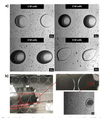
Fig. 4 (a) Influence of the cell concentration on the printability of 4% w/v H2SP-GelMA bio-inks; scale bar = 200  $\mu m$ . (b) Representative images of deposited droplets on tissue culture well plates; the increased probability of nozzle clogging occurs at higher cell concentrations (missing droplet on the left hand side as shown in the enlarged image).
