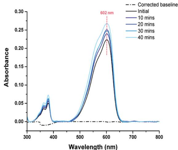
Fig. 3 Overlaid UV-Vis absorbance spectra of aqueous resazurin dye droplets (1 mg per 20 mL), removed from the surface of SiO<sub>2</sub>-PDMS after each 10 minute irradiation interval, up to 40 minutes of UV exposure (254 nm, 8 W). The highlighted absorption peak is at 602 nm, showing that no peak shift has occurred over time. All spectra have been baseline corrected.
