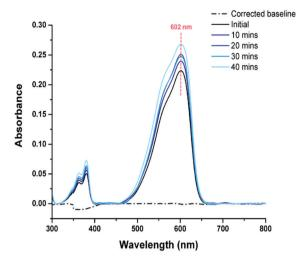
Fig. 3 Overlaid UV-Vis absorbance spectra of aqueous resazurin dye droplets (1 mg per 20 mL), removed from the surface of SiO<sub>2</sub>-PDMS after each 10 minute irradiation interval, up to 40 minutes of UV exposure (254 nm, 8 W). The highlighted absorption peak is at 602 nm, showing that no peak shift has occurred over time. All spectra have been baseline corrected
