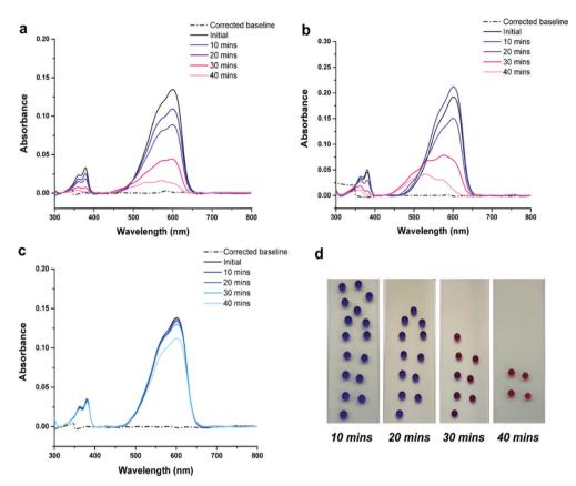
Fig. 4 Overlaid UV-Vis absorbance spectra of aqueous resazurin dye droplets (1 mg per 20 mL), removed from the surface of (a) flat elemental sulfur, (b) PER\_60-60 under standard conditions (254 nm, 8 W) and (c) PER\_60-60 when left in the dark. (d) Digital images of dye droplets on the surface of PER\_60-60 after exposure to 10-40 minutes of UV (left to right, 254 nm). All spectra have been baseline corrected
