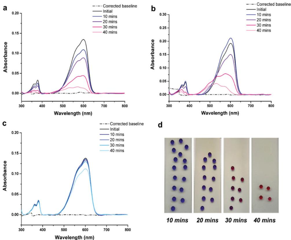
Fig. 4 Overlaid UV-Vis absorbance spectra of aqueous resazurin dye droplets (1 mg per 20 mL), removed from the surface of (a) flat elemental sulfur, (b) PER<sub>60</sub>-60 under standard conditions (254 nm, 8 W) and (c) PER<sub>60</sub>-60 when left in the dark. (d) Digital images of dye droplets on the surface of PER<sub>60</sub>-60 after exposure to 10–40 minutes of UV (left to right, 254 nm). All spectra have been baseline corrected.
