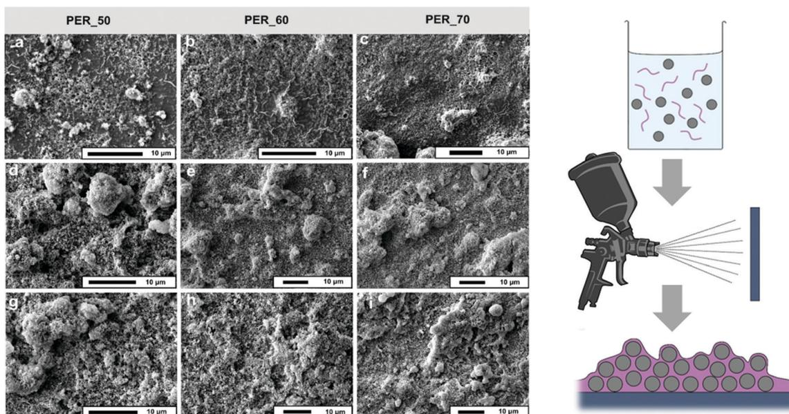
Fig. 2 (a–i) Top-down SEM micrographs showing the morphology of (a) PER<sub>50</sub>-30, (b) PER<sub>60</sub>-30, (c) PER<sub>70</sub>-30, (d) PER<sub>50</sub>-60, (e) PER<sub>60</sub>-60, (f) PER<sub>70</sub>-60, (g) PER<sub>50</sub>-90, (h) PER<sub>60</sub>-90 and (i) PER<sub>70</sub>-90. Scale bars are shown. (j) Schematic of coating on substrate.
