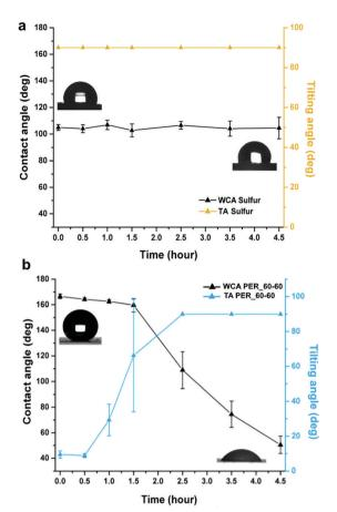
Fig. 5 The change in static contact angle and tilting angle with UV irradiation time (254 nm, 8 W) for (a) sulfur (7 mm diameter pellet, one measurement per pellet, total of 5 readings/pellets per data point) and (b) PER\_60-60. Inset: Corresponding digital image of a water droplet on the surface of sulfur and PER\_60-60 at 0 hours and 4.5 hours.
