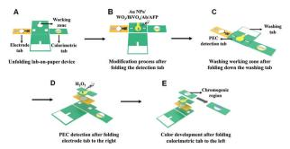
Fig. 1 (A-E) Assembly and operation illustration of the lab-on-paper device. (A) Unfolding the lab-on-paper device. (B) Modification process after folding the detection tab. (C) Washing working zone after folding down the washing tab. (D) PEC detection after folding the electrode tab to the right. (E) Color development after folding the colorimetric tab to the
