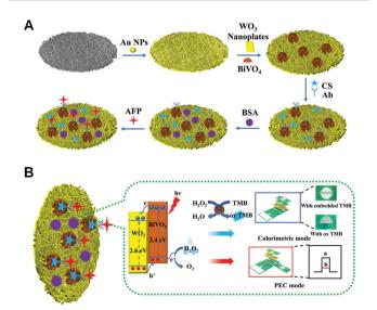
Scheme 1 (A) Fabrication procedure of the lab-on-paper PEC sensing platform. (B) Schematic illustration of the PEC/colorimetric analytical principle. (Colorimetric mode: the folding state of the lab-on-paper device shown in blue rectangle and the colorimetric results before and after incubation of AFP; PEC mode: the folding state of the lab-on-paper device shown in red rectangle and the PEC signal before and after incubation of AFP.)
