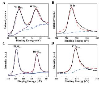
Fig. 3 XPS spectrum of the WO<sub>3</sub>/BiVO<sub>4</sub> heterojunction: (A) W 4f. (B) O 1s. (C) Bi 4f. (D) V 2p.
