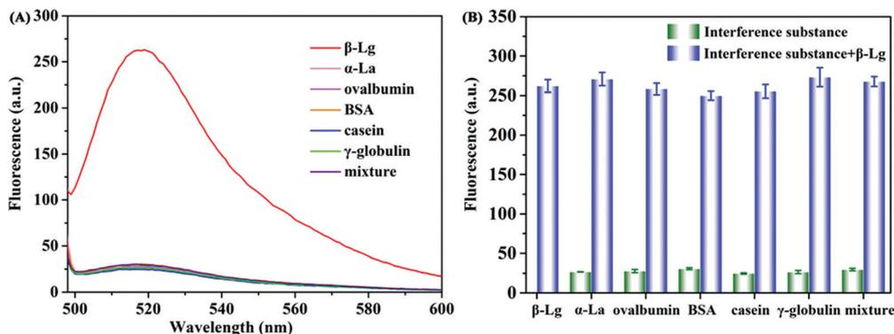
Fig. 5 Selectivity of the method. (A) Fluorescence emission spectra and (B) the fluorescence intensity at 518 nm of the system upon the addition of  $\beta$ -Lg,  $\alpha$ -La, ovalbumin, BSA, casein,  $\gamma$ -globulin and mixture proteins.
