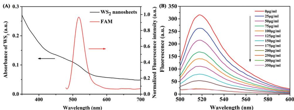
Fig. 2 (A) Spectral overlap between fluorescence emission spectra of FAM fluorescent dye and absorption spectra of  $\text{WS}_2$  nanosheets. (B) The fluorescence spectra of FAM-labelled  $\beta$ -Lg aptamers incubated with different concentrations of  $\text{WS}_2$  nanosheets.
