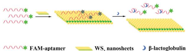
Fig. 1 Schematic diagram for detecting  $\beta$ -Lg based on aptamers and WS<sub>2</sub> nanosheets.
