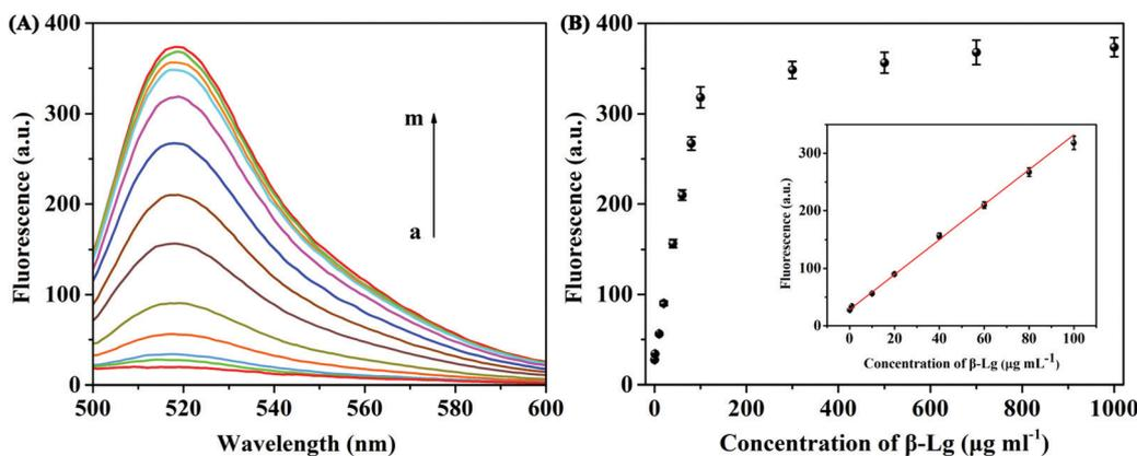
Fig. 4 (A) FAM labelled  $\beta$ -Lg aptamer fluorescence emission spectra of the proposed method at different concentrations of  $\beta$ -Lg ( $0, 0.1, 1, 10, 20, 40, 60, 80, 100, 300, 500, 700,$  and  $1000\ \mu\text{g mL}^{-1}$ ). (B) Diagram of peak fluorescence and target  $\beta$ -Lg concentration. Inset: Linear fitting of fluorescence intensity at 518 nm with the target  $\beta$ -Lg concentration.
