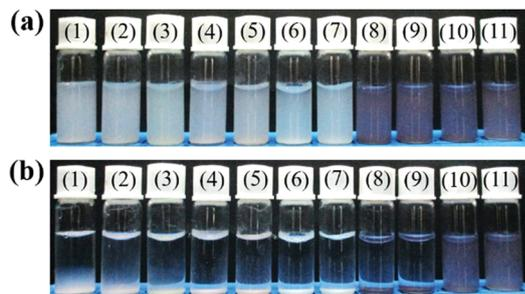
**Fig. 3** Dispersion photographs of poly(4-VP-co-EGDMA) (1), polym@NBD-MIP (2), polym@NBD-CP (3), polym@NBD-MIP@lcPGMA (4), polym@NBD-CP@lcPGMA (5), polym@NBD-MIP@lcPGMA-SH (6), polym@NBD-CP@lcPGMA-SH (7), polym@NBD-MIP@lcPGMA@AuNPs (8), polym@NBD-CP@lcPGMA@AuNPs (9), polym@NBD-MIP@lcPGMA@AuNPs@PHEMA (10), and polym@NBD-CP@lcPGMA@AuNPs@PHEMA (11) in pure water at 25 °C after setting for 0 h (a) and 3 h (b), respectively.
