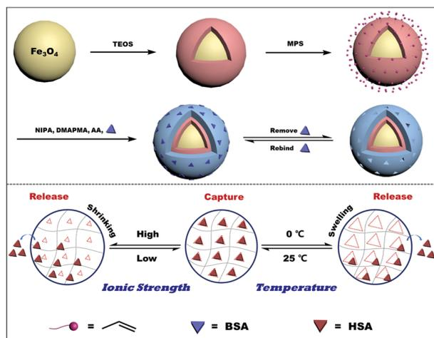
Scheme 1 Schematic illustration for the synthesis of MSR-BSA-MIPs.
