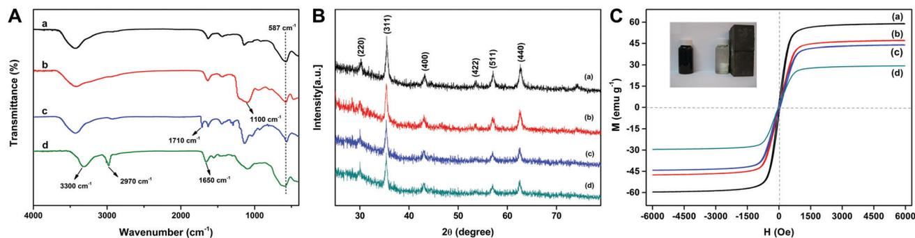
Fig. 3 FT-IR spectra (A), XRD (B), and VSM (C) of Fe<sub>3</sub>O<sub>4</sub> (a), Fe<sub>3</sub>O<sub>4</sub>@SiO<sub>2</sub> (b), Fe<sub>3</sub>O<sub>4</sub>@SiO<sub>2</sub>@MPS (c), and MSR-BSA-MIPs (d).
