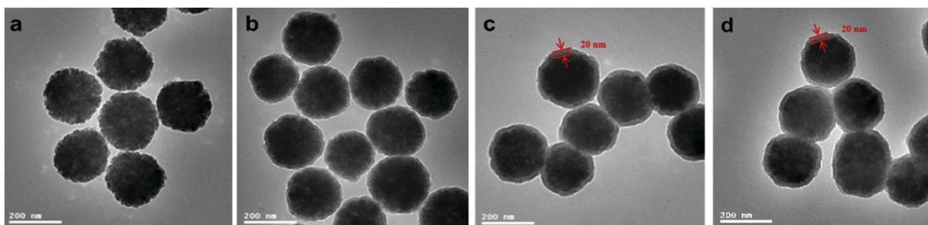
Fig. 2 TEM images of Fe<sub>3</sub>O<sub>4</sub> (a), Fe<sub>3</sub>O<sub>4</sub>@SiO<sub>2</sub> (b), MSR-BSA-MIPs (c), and NIPs (d).
