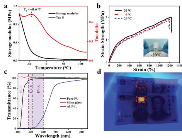
Fig. 6 Characterizations of the ionogel: (a) DMA of the ionogel; (b) strain properties of the ionogel at different temperatures, the insert picture is the stretched ionogel at −20 °C for 1 day storage; (c) the UV absorption of the ionogel; (d) demonstration of the remarkable UV-blocking performance of the ionogel.
