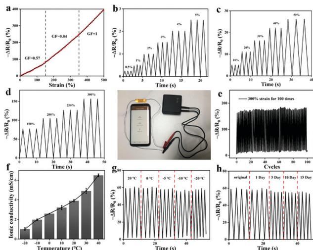
**Fig. 8** The sensing performance of ionogel: (a) the variation of  $\Delta R/R_0$  against the strain (gauge factor); the variation of  $\Delta R/R_0$  at (b) 0.5% to 5%; (c) 5% to 50%; (d) 150% to 300%; (e) 300% for 100 cycles; (f) the conductivities of ionogel at different temperatures; the comparison of the sensing signal at (g) different temperatures; (h) different storage time periods at  $-20^\circ\text{C}$ .
