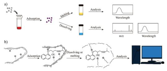
Fig. 6 (a) An elution-free SPE process based on MIW. MIW spheres that adsorbed the target could then be dissolved in n-hexane or melted for subsequent fluorescence and mass spectrum analysis. (b) An overall scheme of target analyte transformation during the SPE process.
