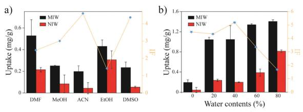
Fig. 3 Optimization of solvents for MIW adsorption towards PRO. (a) The adsorptions of MIW towards PRO (20  $\mu$ g mL<sup>-1</sup>) in different types of solvents. (b) The adsorptions of MIW towards PRO (20  $\mu$ g mL<sup>-1</sup>) in ACN solution with different water contents.
