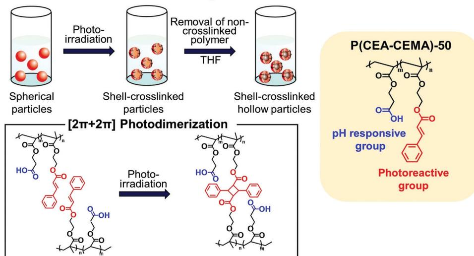
**Scheme 1** Schematic illustration of interfacial photocrosslinking of P(CEA-CEMA)-50 particles for the preparation of hollow particles. pH-responsive release of P(CEA-CEMA)-50 capsule particles. P(CEA-CEMA): poly(2-carboxyethylacrylate-co-2-cinnamoyl ethyl methacrylate).
