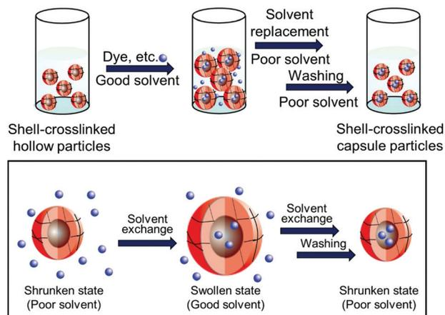
**Scheme 2** Schematic illustration of solvent exchange procedures applied to P(CEA-CEMA)-50 particles for the preparation of capsule particles. P(CEA-CEMA): poly(2-carboxyethylacrylate-co-2-cinnamoyl ethyl methacrylate).
