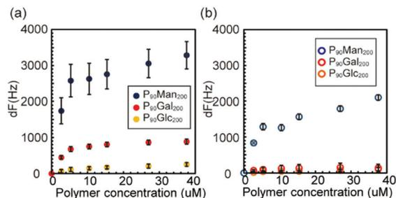
Fig. 3 The frequency change of QCM measurement at each PEG-terminated glycopolymer concentration. (a) Solvent condition; HEPES buffer with  $\text{Ca}^{2+}$  (HEPES: 10 mM, NaCl: 137 mM, KCl: 2.7 mM,  $\text{CaCl}_2$ : 1.8 mM) and (b) HEPES buffer without  $\text{Ca}^{2+}$ .
