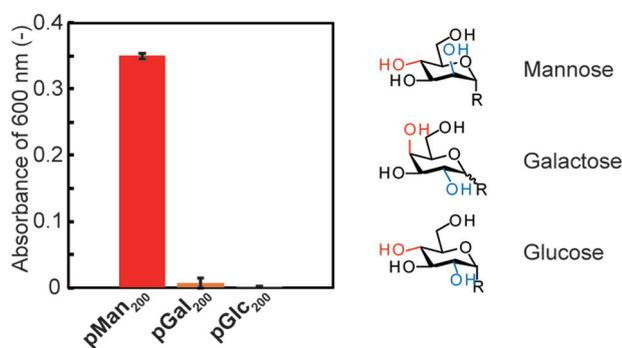
**Fig. 4** Turbidity measurement of **pMan<sub>200</sub>**, **pGal<sub>200</sub>** and **pGlc<sub>200</sub>** and the chemical structure of monosaccharides. Turbidity of each glycopolymer was measured after dissolution in HEPES buffer at  $1 g L^{-1}$  and standing at  $15^\circ C$  for 48 h.
