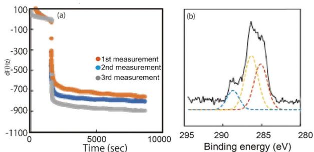
Fig. 2 Glycopolymer layer formation by adsorption of thiol-terminated  $\text{pMan}_{200}$ . (a) Time course of frequency change of three different measurements in QCM by the adsorption of  $\text{pMan}_{200}$  with  $10 \text{ g L}^{-1}$  at  $15 \text{ C}$  for 2 h. (b) XPS C (1s) spectrum of  $\text{pMan}_{200}$  immobilized substrate after the adsorption of the glycopolymer and water rinsing.
