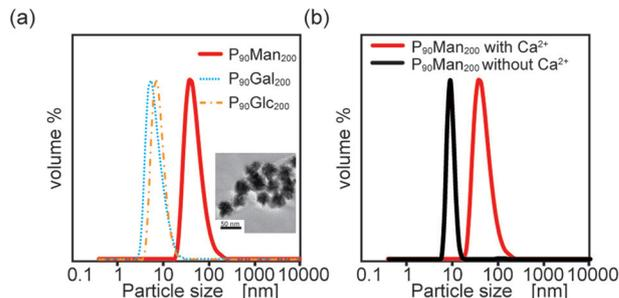
**Fig. 5** (a) DLS measurement of **P<sub>90</sub>Man<sub>200</sub>**, **P<sub>90</sub>Gal<sub>200</sub>** and **P<sub>90</sub>Glc<sub>200</sub>** and the TEM image of **P<sub>90</sub>Man<sub>200</sub>** (inset). (b) DLS measurement of **P<sub>90</sub>Man<sub>200</sub>** with (red) and without (black)  $Ca^{2+}$ .
